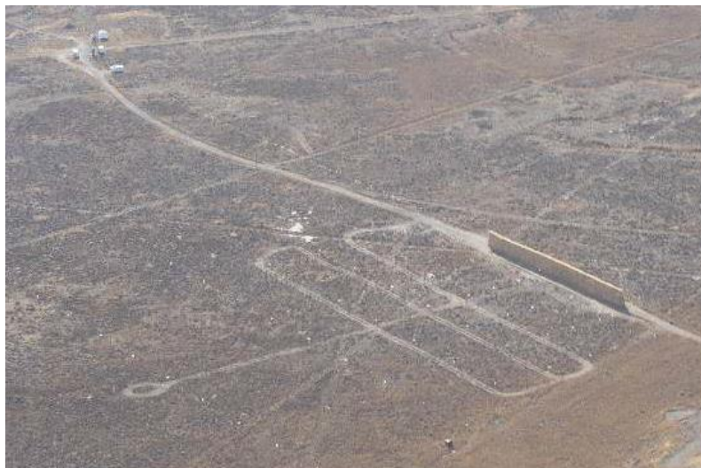
Figure 1 Aerial view of the mock sound barrier (built of 300 1-ton straw bales, 6m in height, 90m in length) test site. In the upper left of the picture, the command center and the release trailer are visible (Source: Figure 5 of Clawson et al. 2009)
