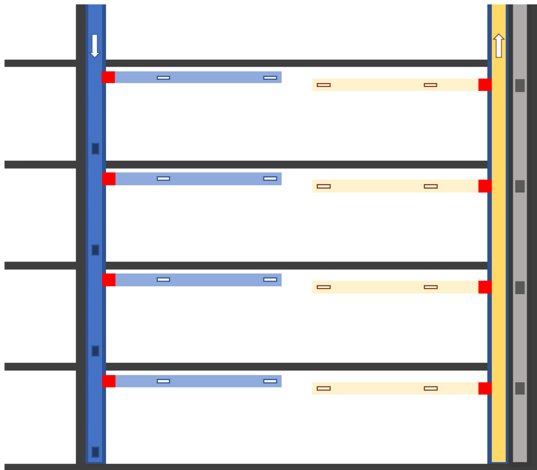
Figure 3 Schematic layout of the ventilation system in one redundant train of the electrical building
