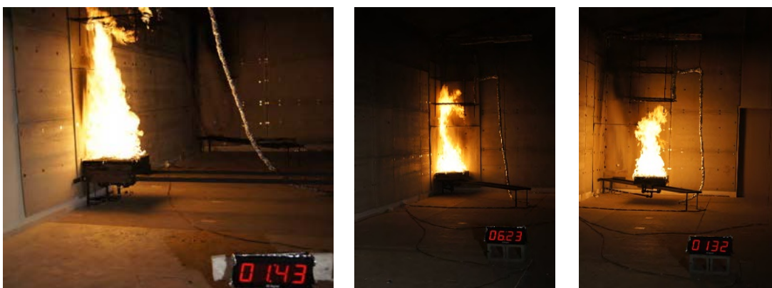
Figure 2 Photographs of burners used for wall and corner tests showing burners located against wall (left), in corner (middle), and moved 0.3 m (1 ft) away from corner (right)
