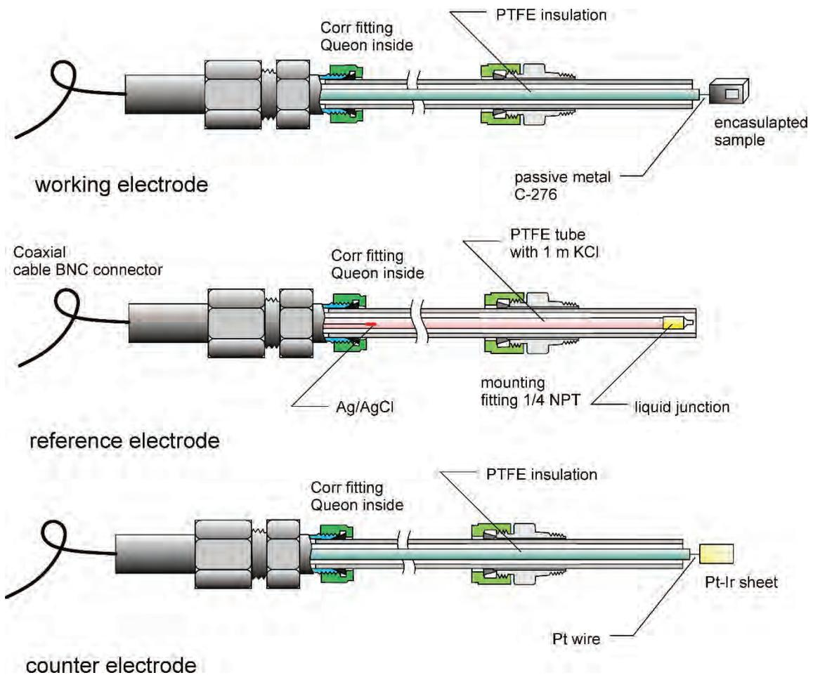
**Fig. 2.2** High-pressure, high-temperature electrodes used for electrochemical experiments
