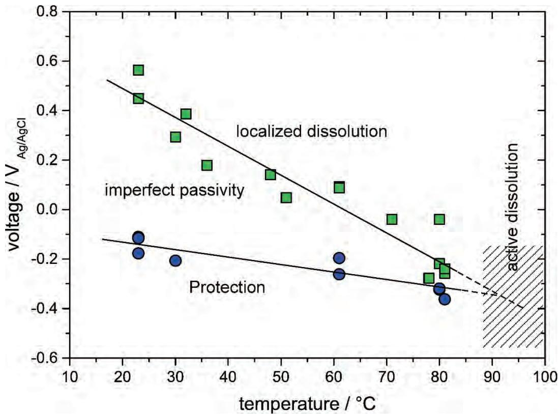
**Fig. 3.2** Breakdown (green) and repassivation potentials (blue) measured at different temperatures on polarization experiments at  $0.001 \text{ V s}^{-1}$  in Q3 solution and  $p = 6 \text{ bar}$
