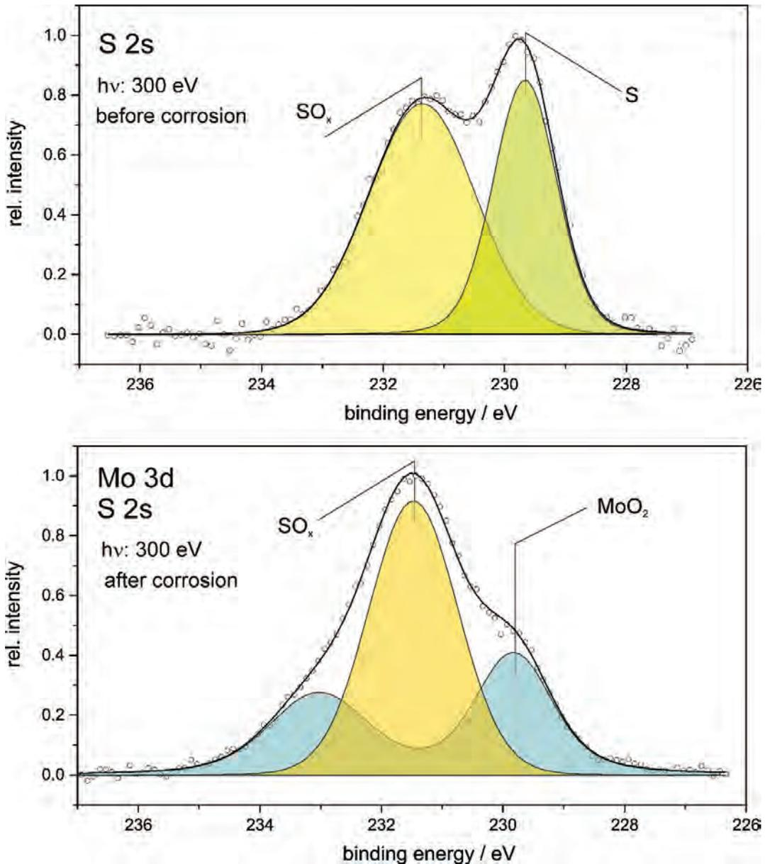
**Fig. 8.11** Mo 3d and S 2s core level spectra of the 309S surface before and after the polarization experiment. Excitation energy: 300 eV
