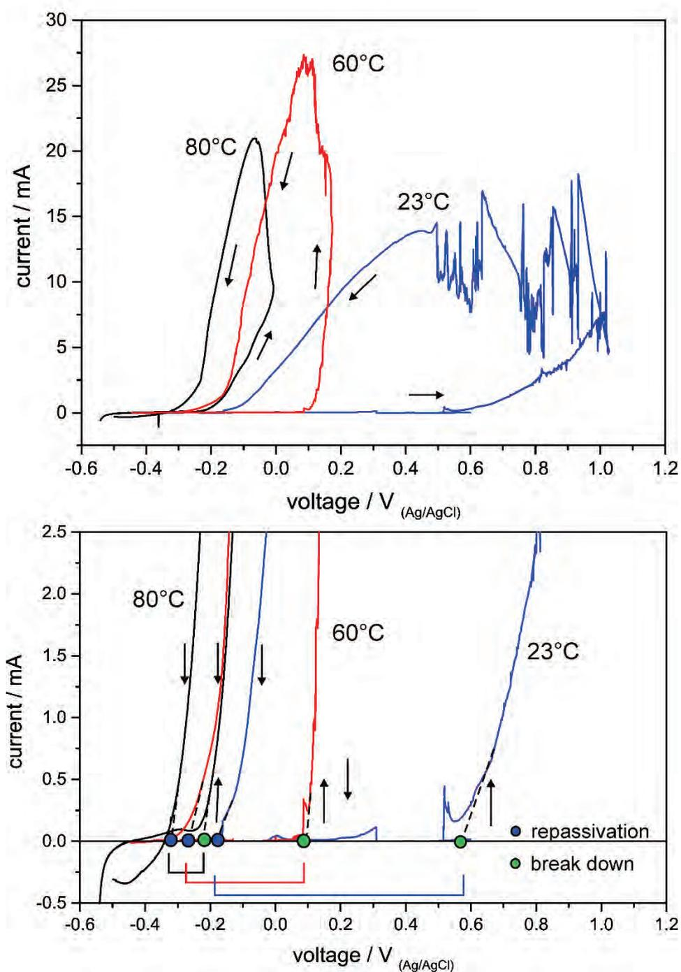
**Fig. 3.1** Linear polarization of steel 309S in Q3 solution at different temperatures and at 3-6 bar pressure. Scan rate: 0.001 V s<sup>-1</sup>
