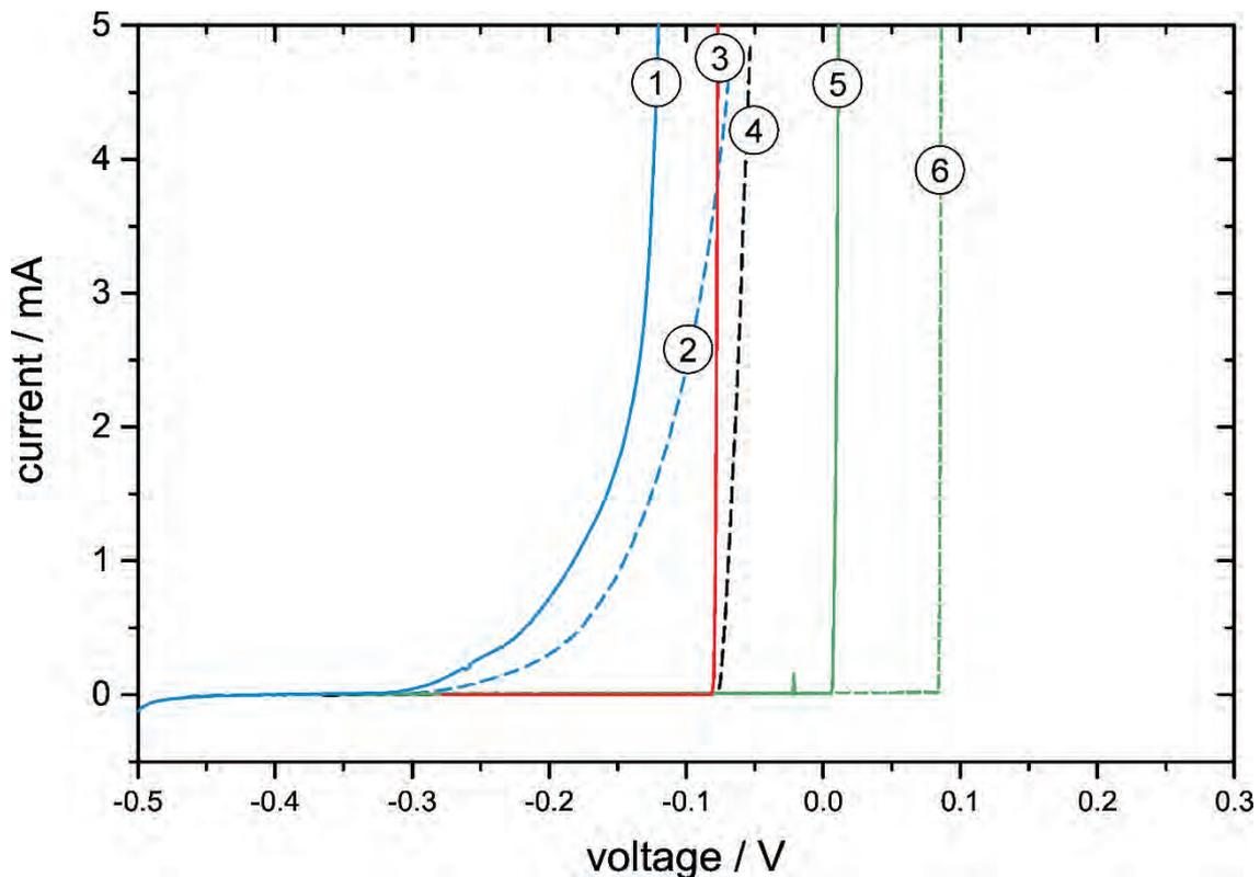
**Fig. 3.17** Polarization curves performed on 309S steel in Q3 solution at 80 °C at different pressures and sample pre-heating programs. Scan rate: 1 mV s<sup>-1</sup>.
