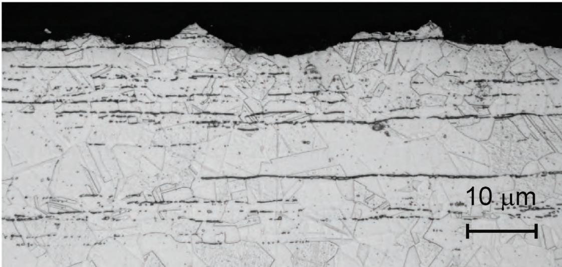
**Fig. 3.16** Light microscopy picture showing a cross section view of a cut performed on a sample after a cyclic polarization at 80 °C and p = 5 bar in Q3 solution. The cut surface was previously polished and etched with V2A solution (10:10:1 water, hydrochloric acid, nitric acid)
