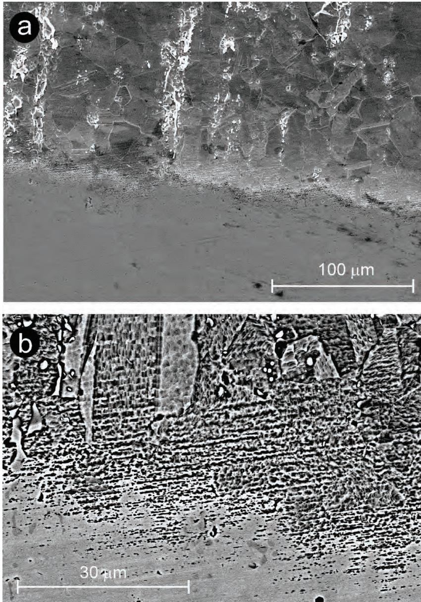
**Fig. 3.8** SEM photographs depicting a magnification of the ribbon shaped corroded area of 309S steel in Q3 solution at 90 °C and  $p = 5$  bar. a: combined material contrast and surface topography; b: material contrast
