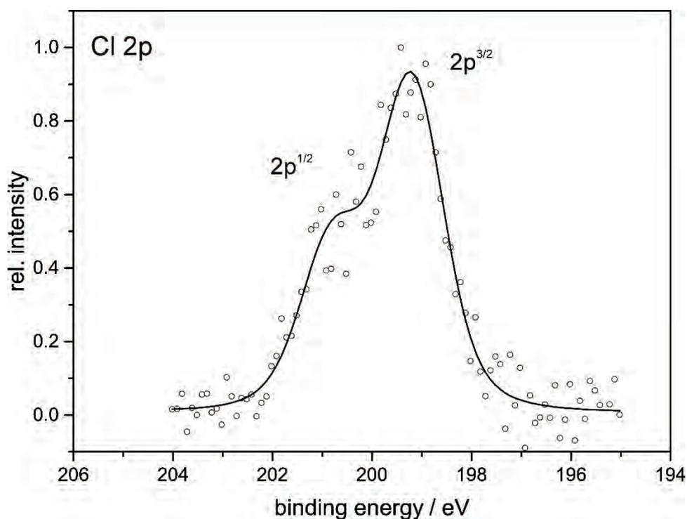
**Fig. 5.14** Cl 2p core level spectrum for the surface inside corroded area after the anodic polarization 6 shown in Fig. 3.17 in Q3 solution at 80 °C and 50 bar
