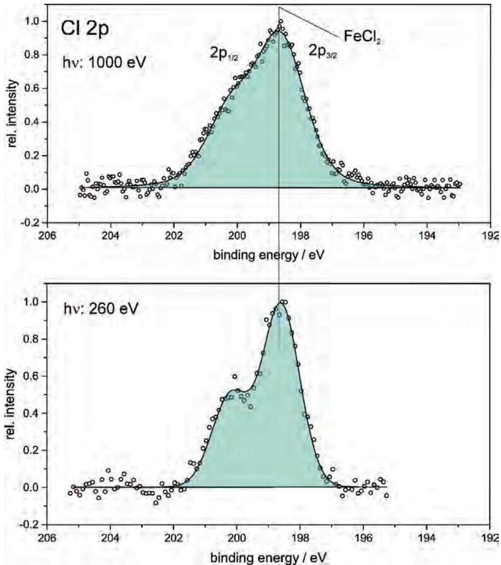
**Fig. 8.6** Cl 2p core level spectra of the 309S surface after the polarization experiment at different excitation energies
