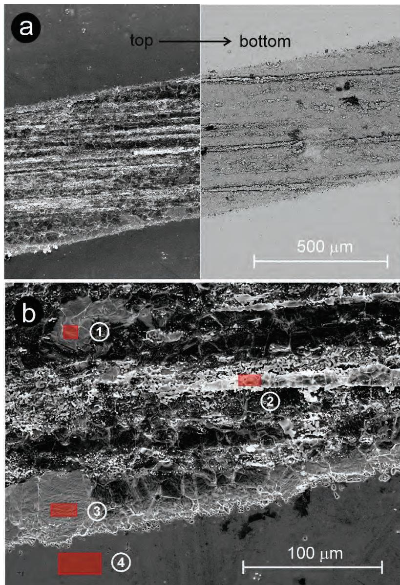
**Fig. 3.11** a: SEM image of 309S steel surface after a cyclic polarization in Q3 solution at 80 °C and  $p = 5$  bar. Left: combined ETD mode, right: material contrast. The position of the electrode during the experiment is indicated; b: magnification of the upper picture a) with indication of points of EDX analysis
