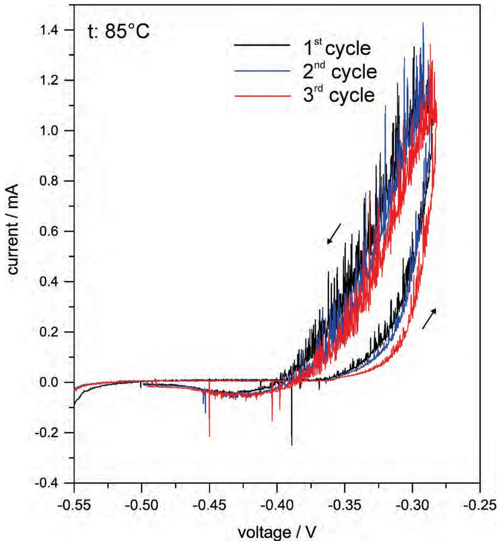
**Fig. 4.2** Cyclic current-voltage curves of 309S steel in Q2 solution at 85 °C. Scan rate: 1 mV s<sup>-1</sup>. Polarization were started at -0.2 V from the OCP. Arrows indicate the scan direction
