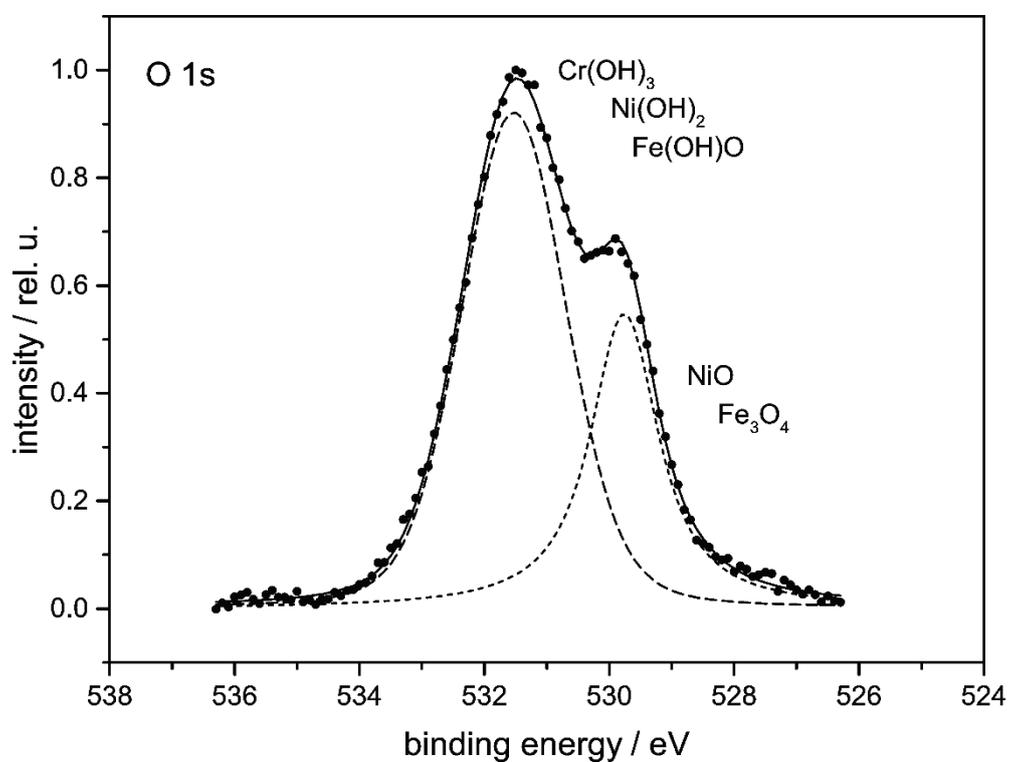
**Fig. 5.12** O 1s core level signal for the surface outside pits after a cyclic polarization in Q3 solution at 23 °C (spectrum corrected by charge)
