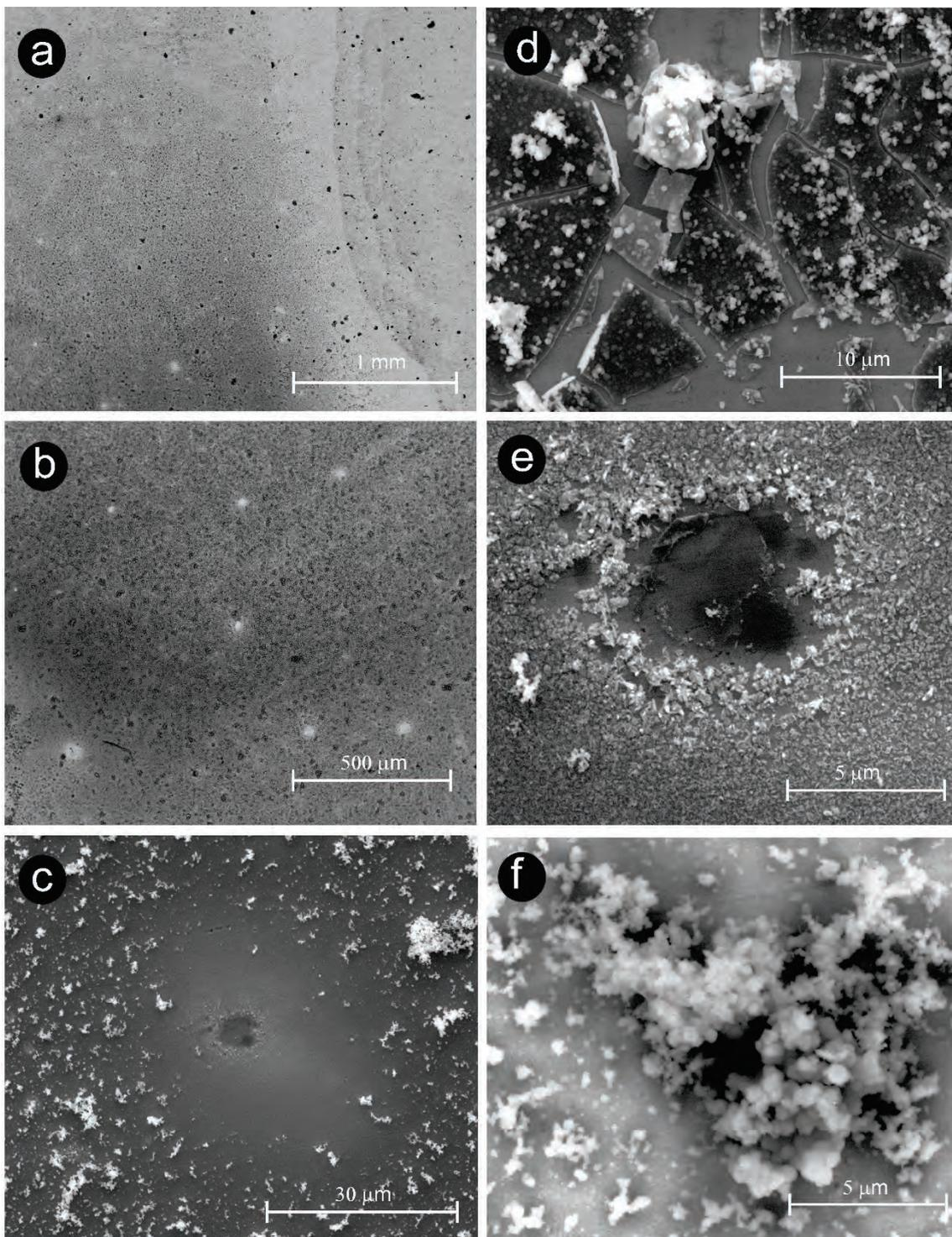
**Fig. 6.5** SEM images at different scales showing the surface of 309S steel after immersion in Q3 solution at 80 °C and 5 bar during 24 h. a) and b) height mode; c), d), e) and f) secondary electron (SE) mode
