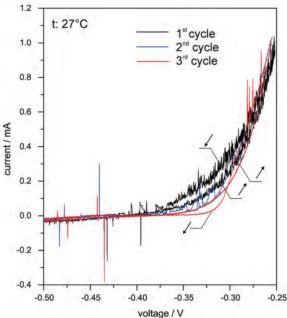
**Fig. 4.1** Cyclic current-voltage curves of 309S steel in Q2 solution at 27 °C. Scan rate:  $1 \text{ mV s}^{-1}$ . Polarization were started at -0.2 V from the OCP. Arrows indicate the scan direction
