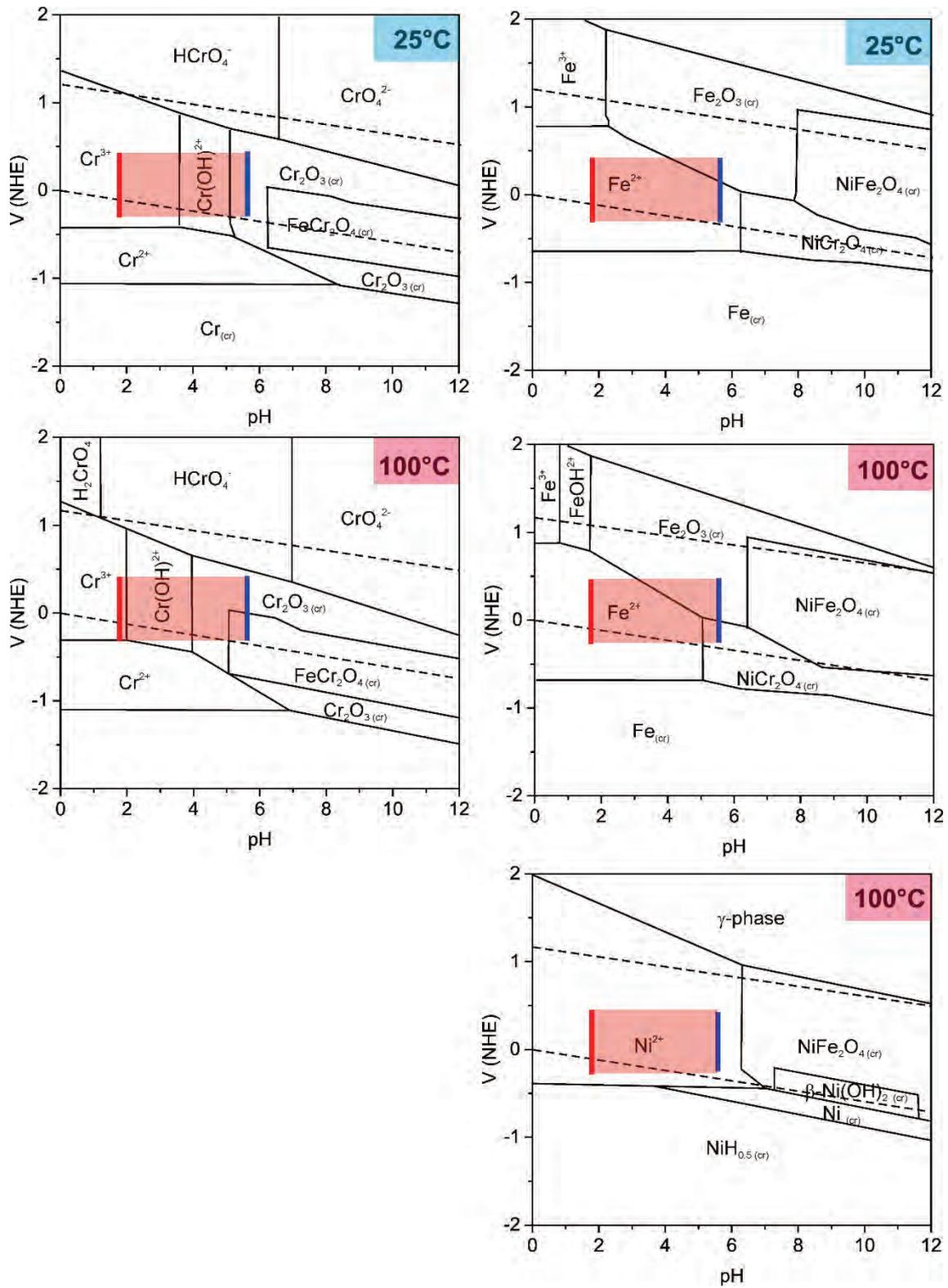
**Fig. 4.6** Pourbaix diagrams for the ternary system Fe-Cr-Ni at 25 °C and 100 °C.  $[\text{Fe}(\text{aq})] = [\text{Cr}(\text{aq})] = [\text{Ni}(\text{aq})] = 10^{-6} \text{ mol kg}^{-1}$  (adapted from /BEV 1999/)
