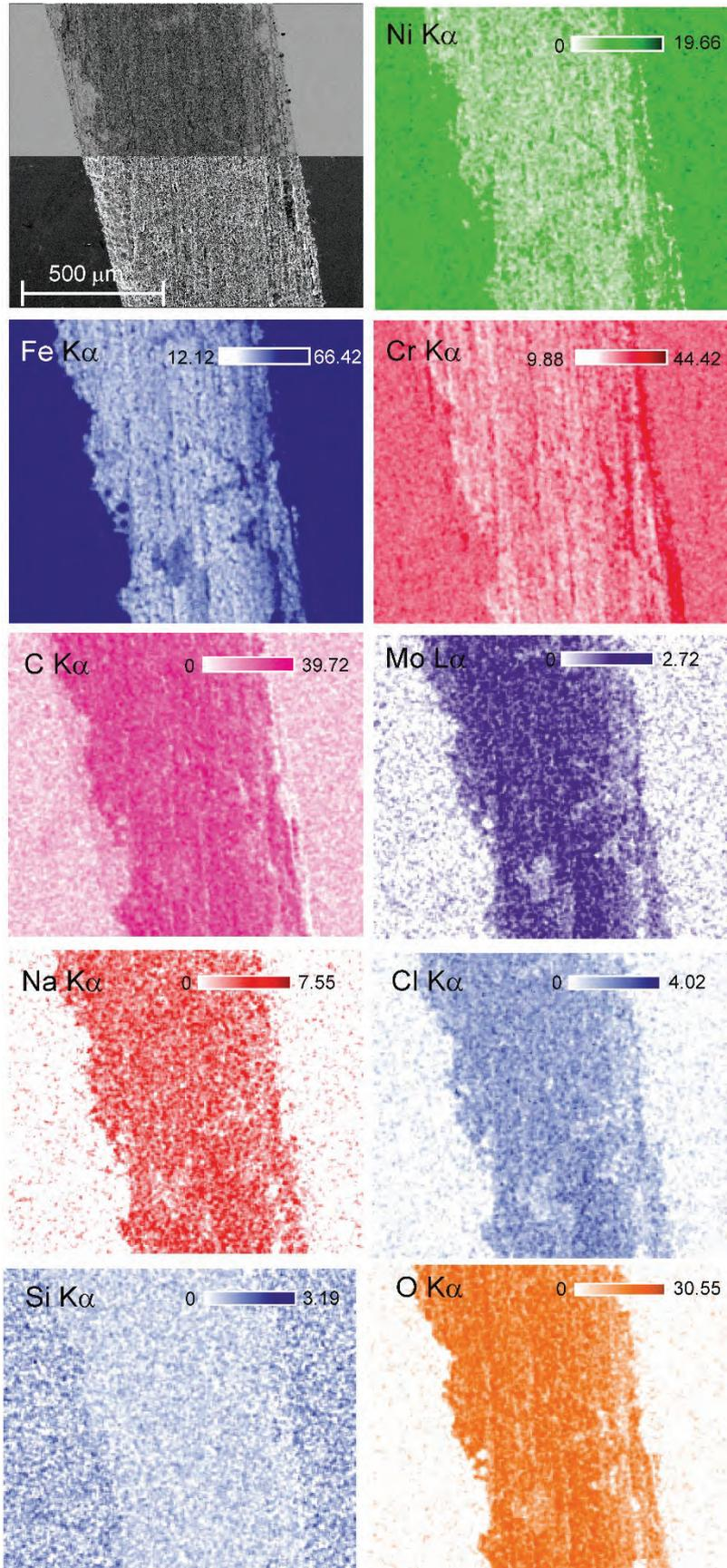
**Fig. 3.12** EDX mapping analysis of a ribbon-type pit observed on 309S steel after a cyclic polarization in Q3 solution at 61 °C and  $p = 6$  bar
