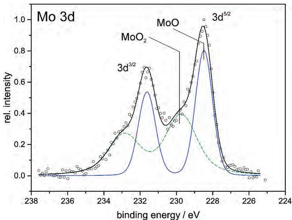
**Fig. 5.13** Mo 3d core level signal for the surface inside corroded area after the anodic polarization 6 shown in Fig. 3.17 in Q3 solution at 80 °C and 50 bar
