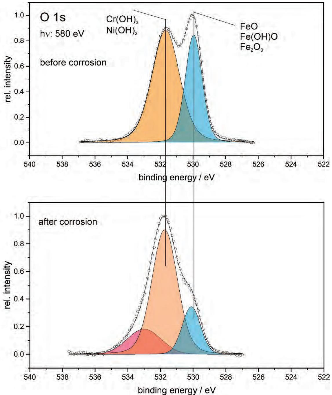
**Fig. 8.5** O 1s core level spectra of the 309S surface before and after the polarization experiment. Excitation energy: 580 eV
