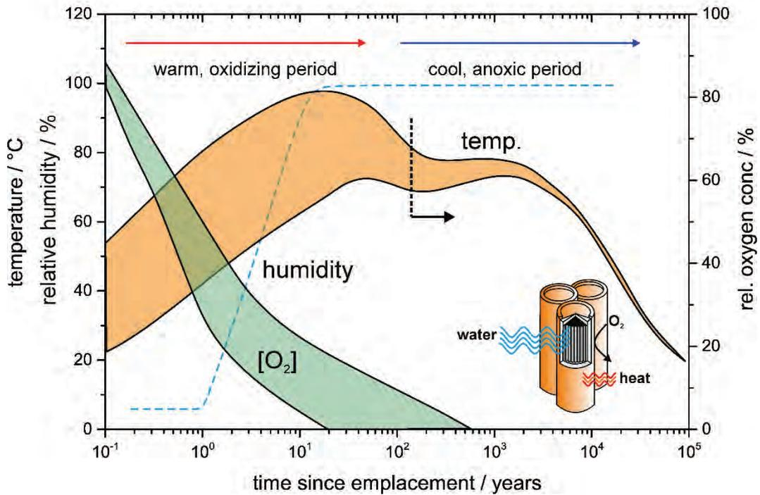
**Fig. 1.2** Schematic evolution of the near-field environment of a repository (after /SHO 2006/)
