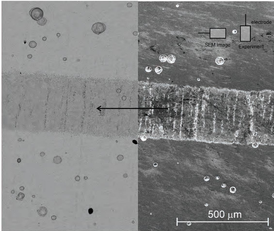
**Fig. 3.7** SEM image of 309S steel surface after a cyclic polarization in Q3 solution at 90 °C and  $p = 5$  bar. Left: backscattered electron image (material contrast), right: combined secondary electron and backscattered electron image (surface topography and material contrast). Arrow indicates the up-down direction of the electrode face during experiment (see scheme at the upper-right corner)
