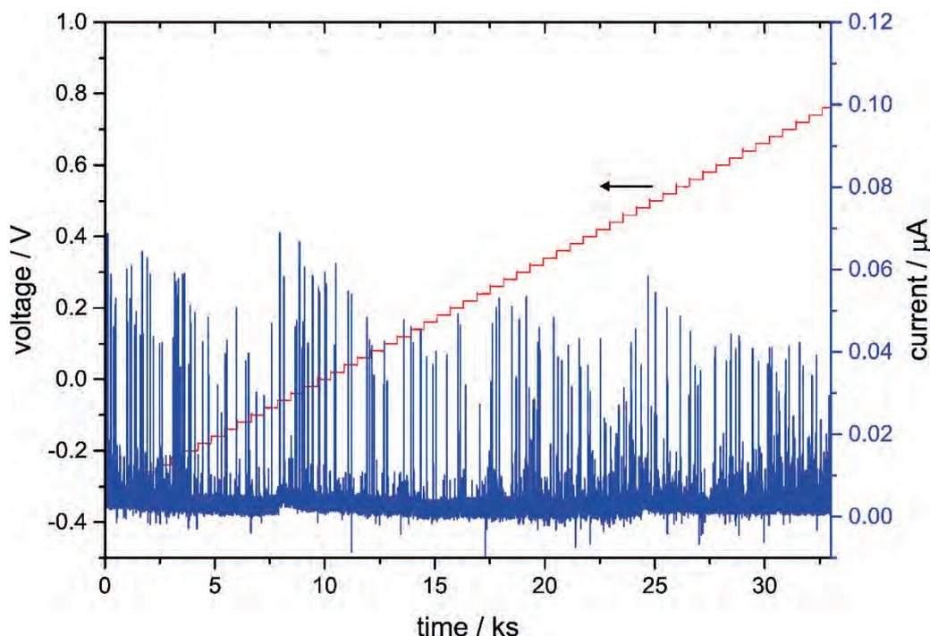
**Fig. 6.1** Temporal evolution of current with a slow staircase voltage scan (step: 20 mV each 10 min) of 309S steel in Q3 solution at 30 °C and 5 bar.  $V_i$  = OCP (open circuit potential)
