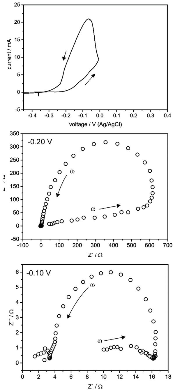
**Fig. 7.3** Nyquist plots obtained at different potentials after a cyclic polarization of 309S steel in Q3 solution at 80 °C and  $p = 6$  bar (current-voltage curve shown at the top-left corner: scan rate  $1 \text{ mV s}^{-1}$ ). Frequency range: 1 MHz – 30 mHz. Amplitude: 10 mV
