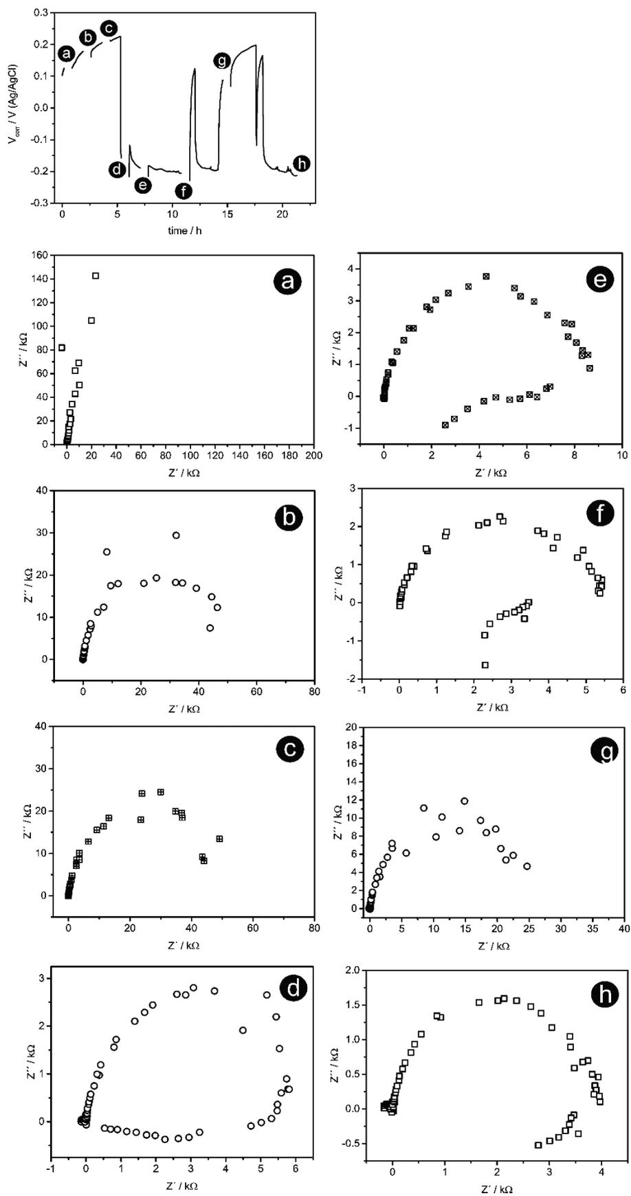
**Fig. 7.5** Nyquist plots performed at the corrosion voltage at regular time intervals with a 24 h test in Q3 solution at 30 °C and 6 bar
