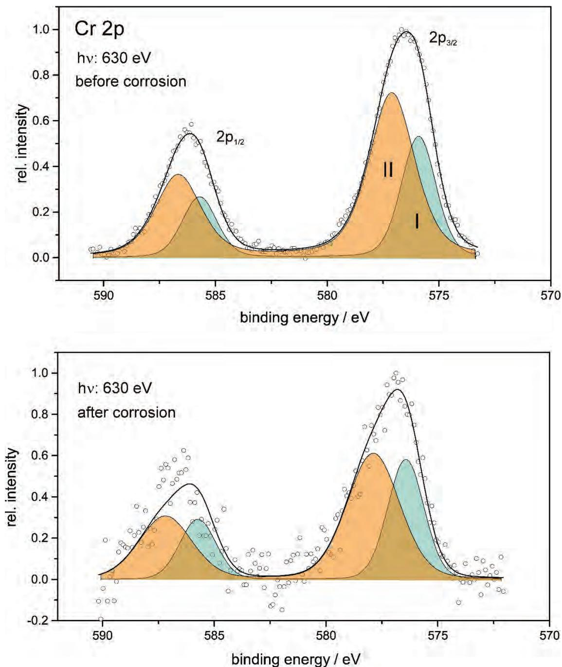
**Fig. 8.8** Cr 2p core level spectra of the 309S surface before and after the polarization experiment. Excitation energy: 630 eV
