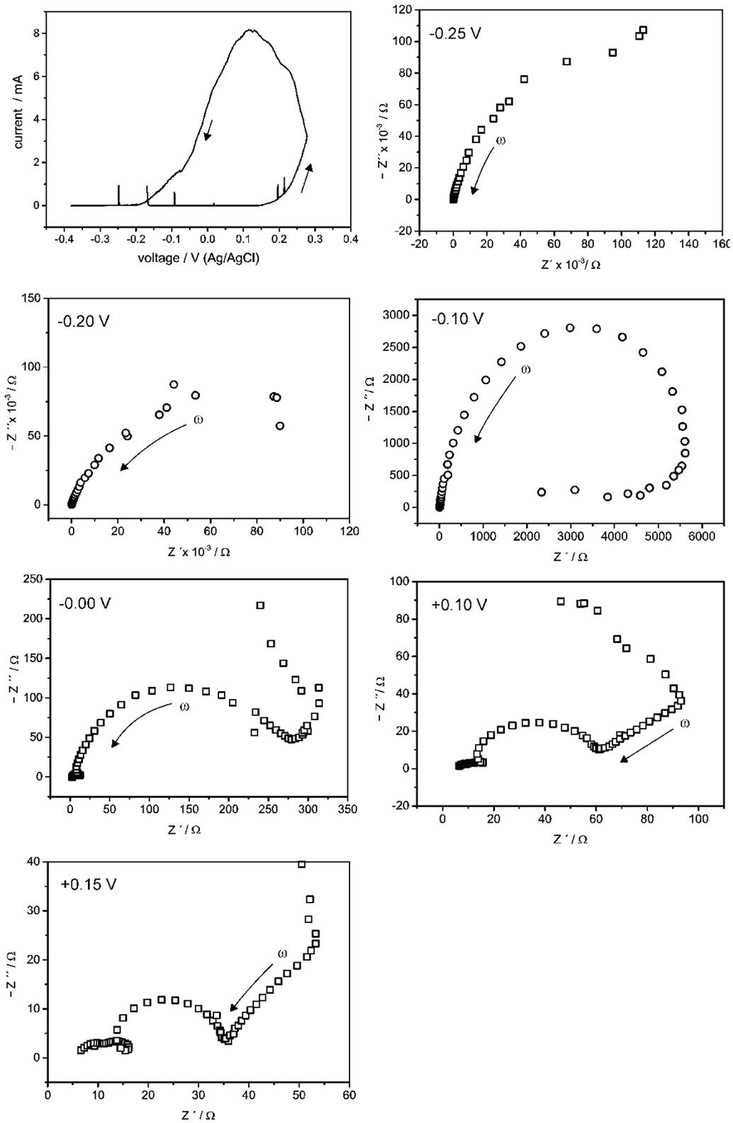
**Fig. 7.2** Nyquist plots obtained at different potentials after a cyclic polarization of 309S steel in Q3 solution at 30 °C and  $p = 6$  bar (current-voltage curve shown at the top-left corner: scan rate 1 mV s<sup>-1</sup>). Frequency range: 1 MHz – 30 mHz. Amplitude: 10 mV
