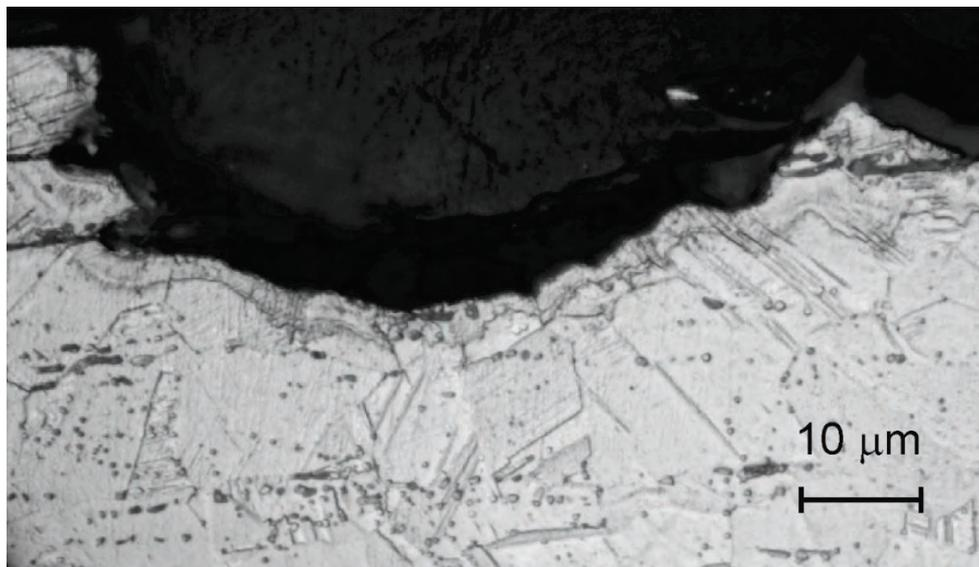
**Fig. 3.6** Light microscopy picture showing a cross section view of a cut performed on a corroded sample. The cut surface was previously polished and etched with V2A solution (10:10:1 water, hydrochloric acid, nitric acid)
