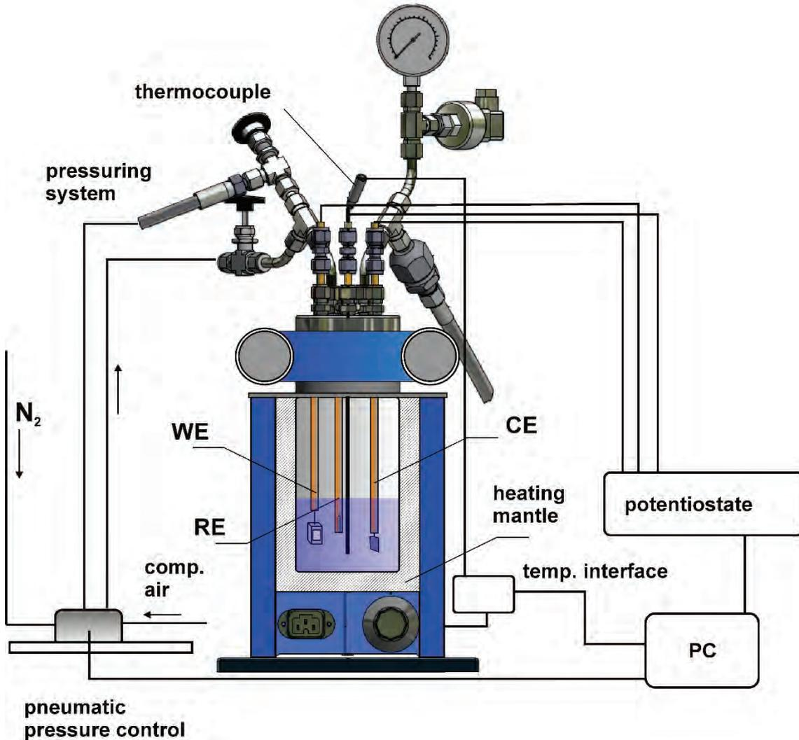
**Fig. 2.1** Schematic showing the high-temperature, high-pressure electrochemical cell system for corrosion studies. WE: working electrode; CE: counter electrode; RE: reference electrode
