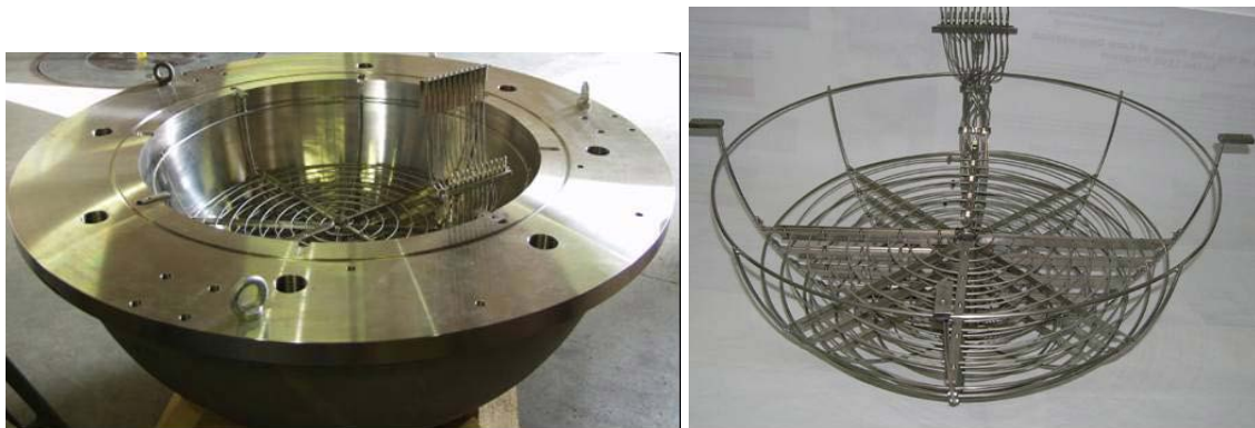
Fig. 5.89 Test vessel with the volumetric heating system /GAU 11/
