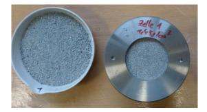
a. bentonite specimens placed in a bowl and confined in a cell
