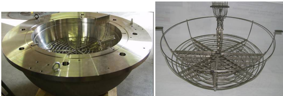
Fig. 5.87 Test vessel with the volumetric heating system /GAU 11/
