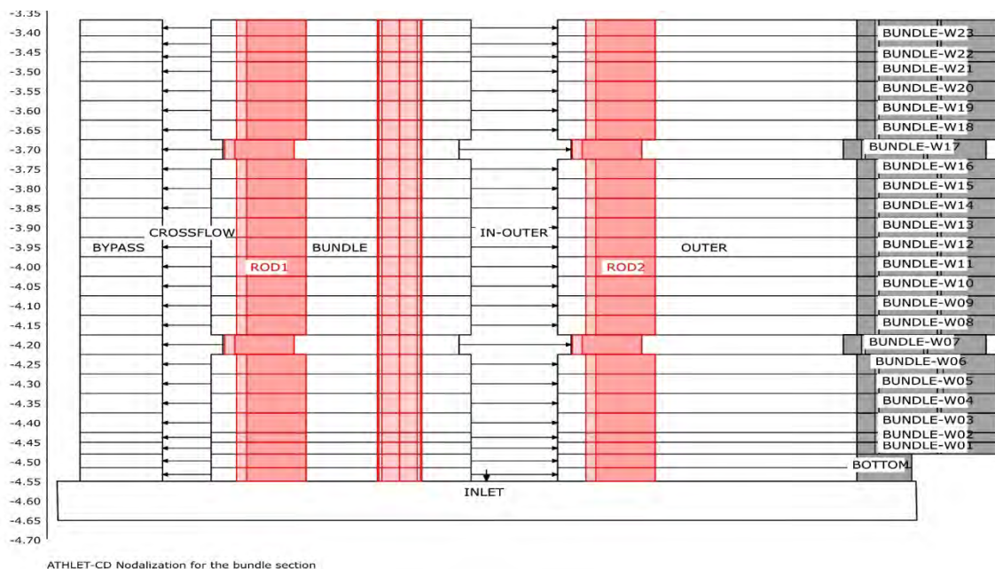
Fig. 5.30 ATHLET-CD Nodalisation for PHEBUS test FPT1 (bundle)
