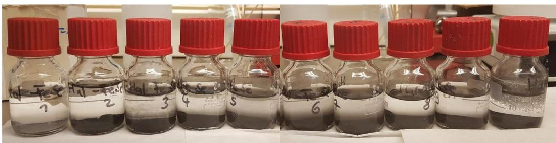
**Fig. 8.10** Experimental batches of FeSe in halite/ anhydrite-saturated solution
