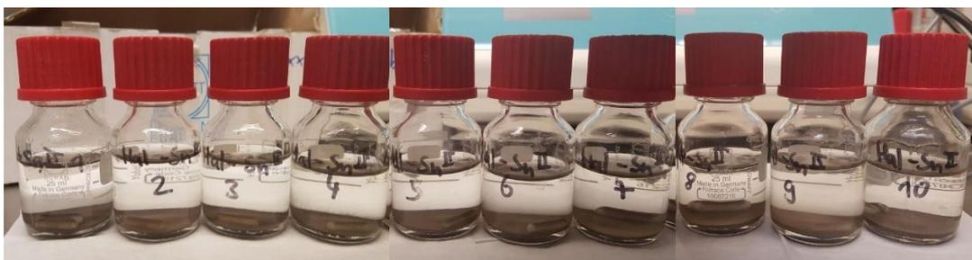
**Fig. 8.15** Experimental batches of tin(II) in halite/ anhydrite-saturated solution
