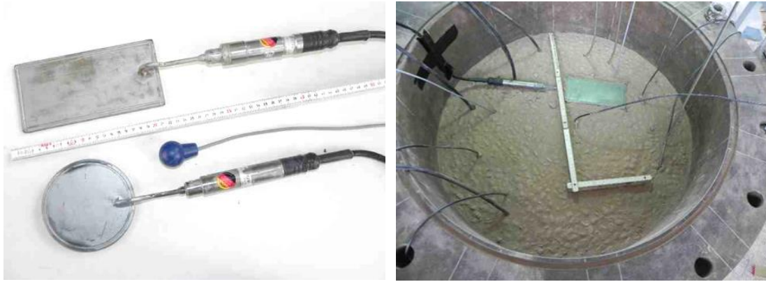
Fig. 5.39 Surface pressure transducers (left) from GLÖTZL for measurement in axial direction (top), in radial direction (bottom), pressure transducer from KELLER for non-directional measurement (middle) and axial surface pressure transducer P6 on top of the DS4 in HTV-8 (right)
