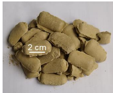
Calcigel, HTV-7 \rho_{d,105\text{ °C}} = 1.91\text{ g/cm}^3
