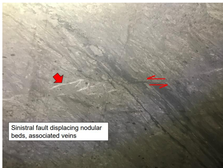
Fig. 3.20 Fault with sinistral shear displacing a nodular sedimentary layer by about 2 cm. On the left-hand side, there are conjugated Calcite veins occurring (Photo by D. Jaeggi, swisstopo)
