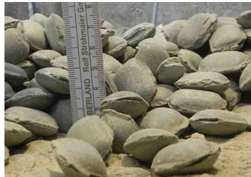
Fig. E. 1 Bentonite pillows in binary mixture of DS during installation of HTV-7 to HTV-9
