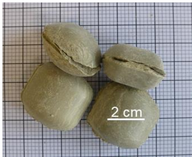
Calcigel, HTV-5 \rho_{d,105\text{ °C}} = 1.98\text{g/cm}^3
