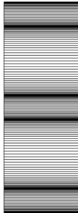
Fig. 6.10 Mesh used for the COMSOL model of MiniSandwich Test 8
