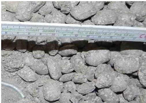
Fig. E. 1 Bentonite pillows in binary mixture of DS during installation of HTV-7 to HTV-9
