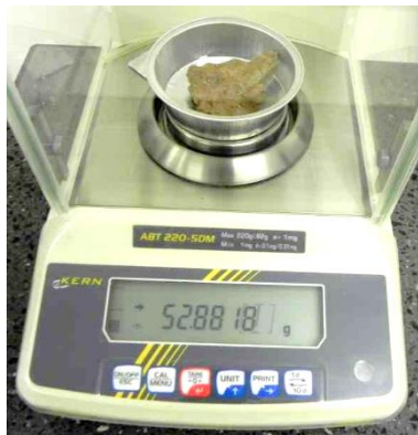
Fig. B. 3 Weighing M1 of a bentonite sample for density determination in air
