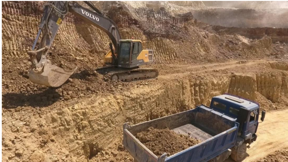
Fig. 5.8 Excavation and transport of plastic clay F1623 in the Meudt mine
