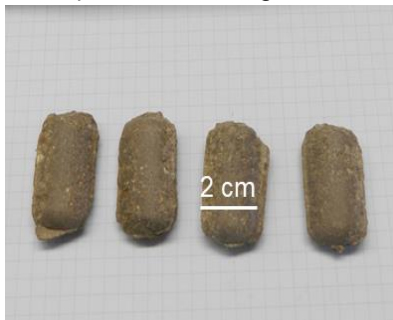
Secursol UHP, HTV-6 \rho_{d,105\text{ °C}} = 1.91\text{g/cm}^3
