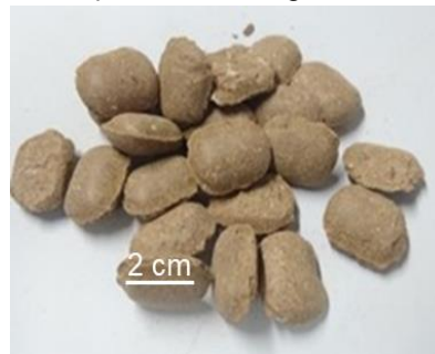
Secursol MHP1 (70/30), HTV-8 \rho_{d,105\text{ °C}} = 1.93\text{ g/cm}^3
