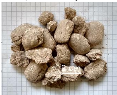
Secursol MHP1 (70/30), Shaft 2, HTV-9 \rho_{d,105\text{ °C}} = 1.87\text{g/cm}^3
