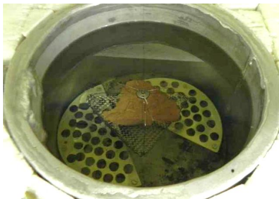
Fig. B. 4 Weighing M2 of a bentonite sample for density determination in silicone oil ELBESIL B10
