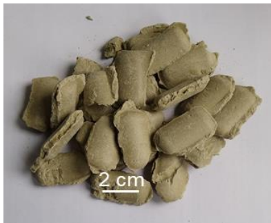
Calcigel, Shaft 1 \rho_{d,105\text{ °C}} = 1.70^*\text{ g/cm}^3
