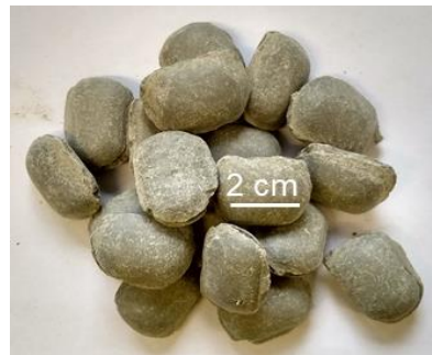
Calcigel, Shaft 2 and HTV-9 \rho_{d,105\text{ °C}} = 2.05\text{ g/cm}^3
