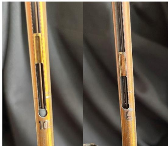
**Fig. 2** ORANO temperature sensors composed of bimetallic washers inside a stainless-steel tube.
