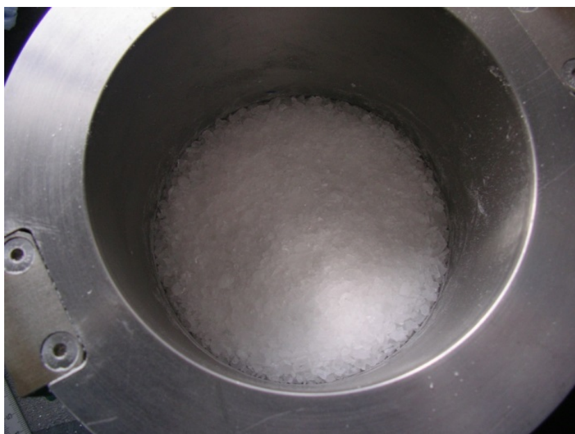
Fig. 3.2 Crushed salt in the test cell
