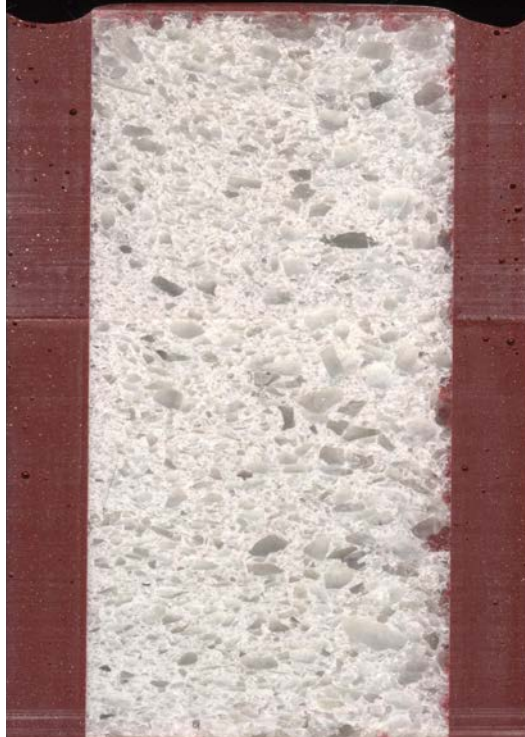
Fig. F.6 Intrusion of coloured resin into the pore space of a compacted sample
