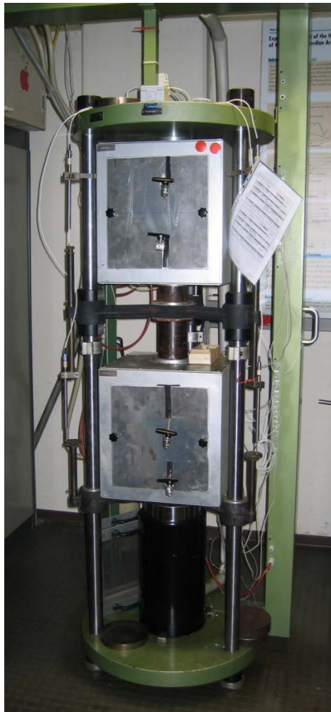
Fig. 2.3 Frame of the testing machine holding two test chambers
