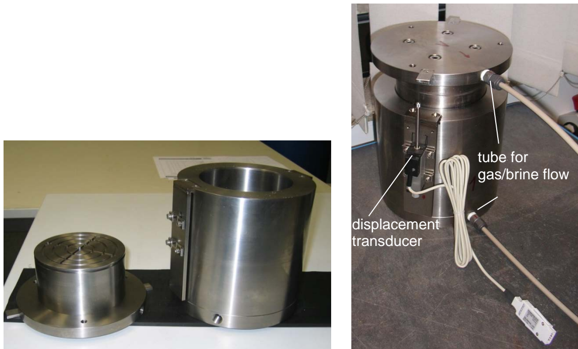
Fig. 2.1 Test cell; left: open and empty, right: ready for the test
