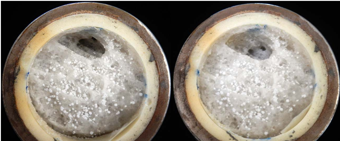
Fig. F.12 Top and bottom of sample M2a after some dissolution in boiling water.
