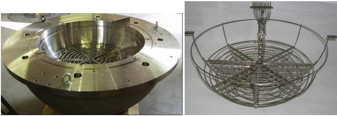
Fig. 5.82 Test vessel with the volumetric heating system /GAU 11/
