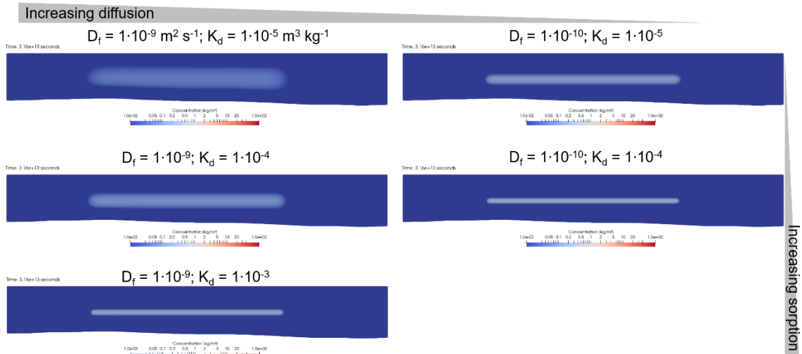
Figure 42: Concentration distribution for different diffusion coefficients ( 1 \cdot 10^{-9}, 1 \cdot 10^{-10} \text{ m}^2 \text{ s}^{-1} ) and different sorption coefficients ( K_d -value: 1 \cdot 10^{-5}, 1 \cdot 10^{-4}, 1 \cdot 10^{-3} \text{ m}^3 \text{ kg}^{-1} ) after 1 million years.
