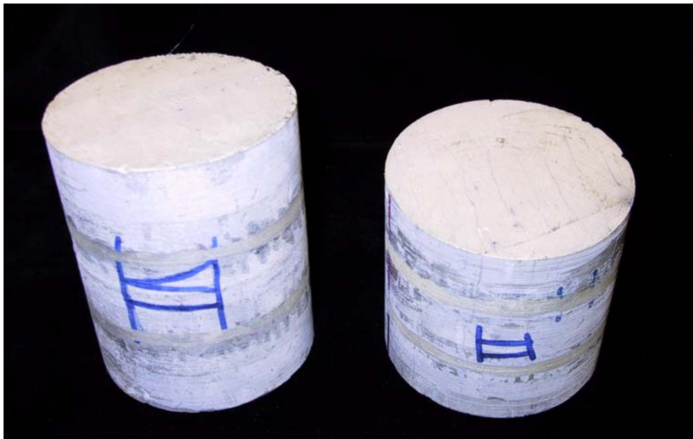
Figure 4-8 Prepared samples with conductive silver lacquer at the end surfaces and rings over the circumference
