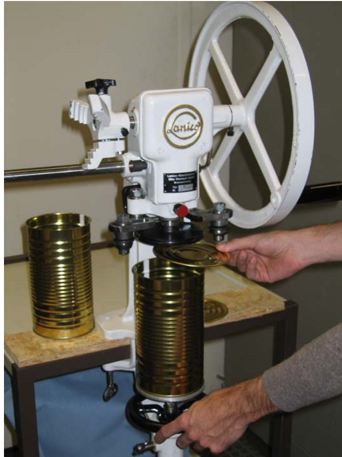
Figure 4-12 Folding machine for tin boxes with tin boxes of 113 mm diameter and 205 mm height
