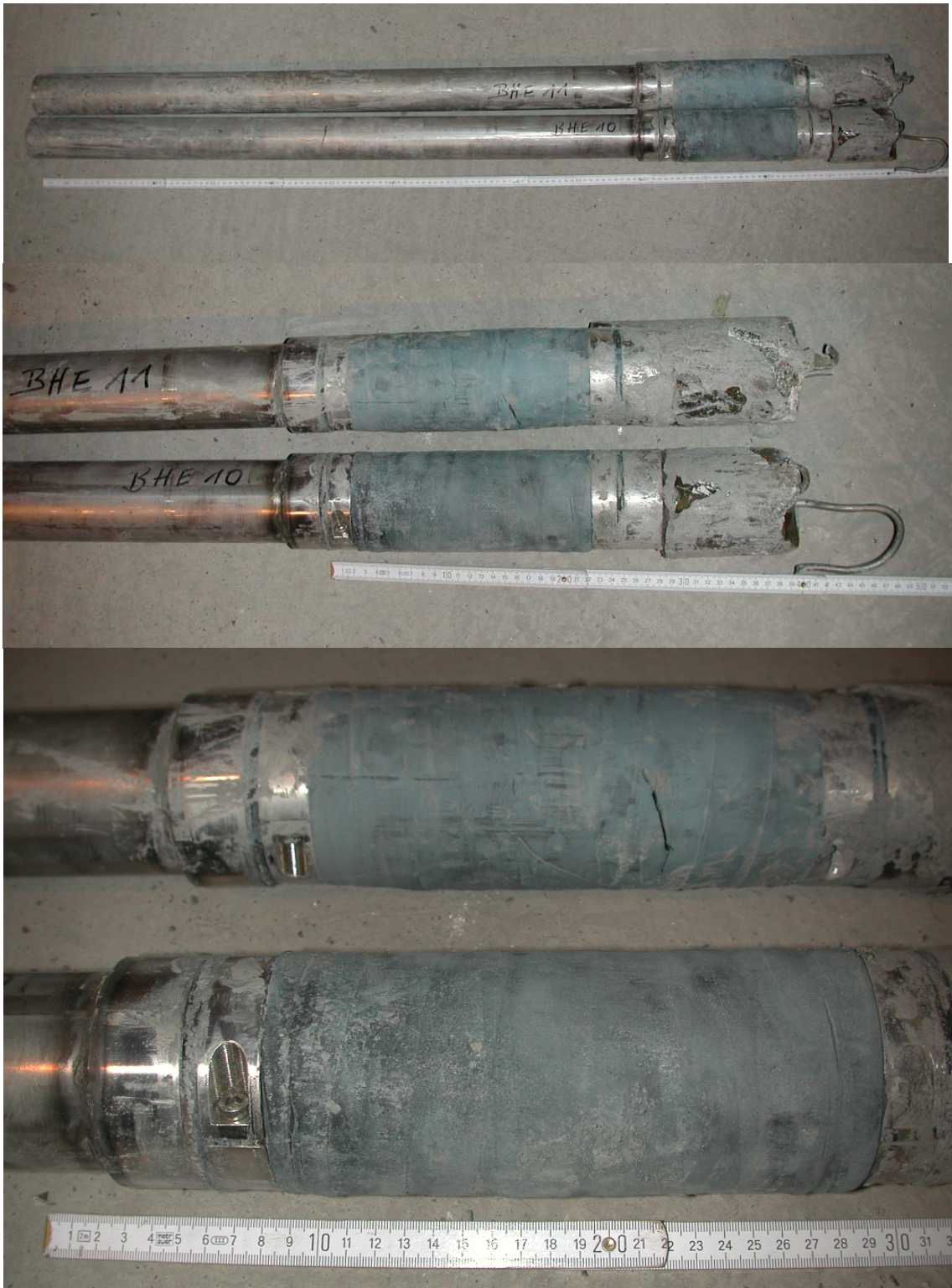
Figure 5-23 Dismantled packers from the boreholes BHE-10 and BHE-11
