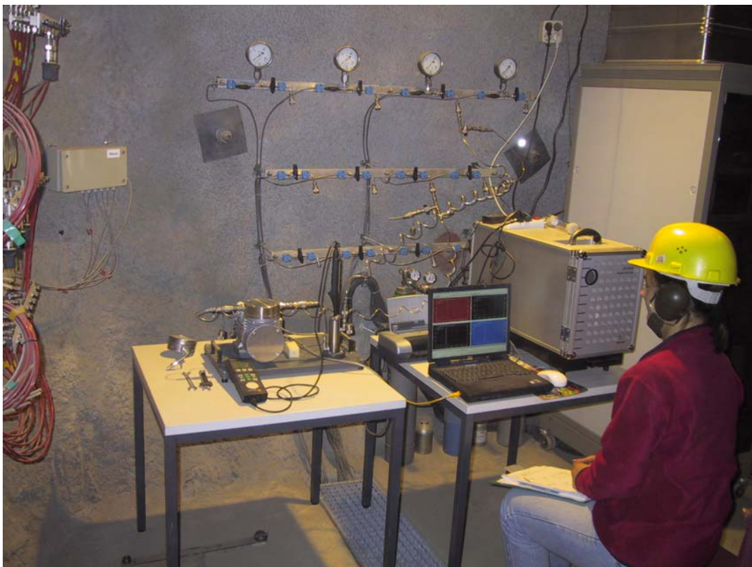
Figure 4-3 Gas chromatograph in operation in the HE-B test field
