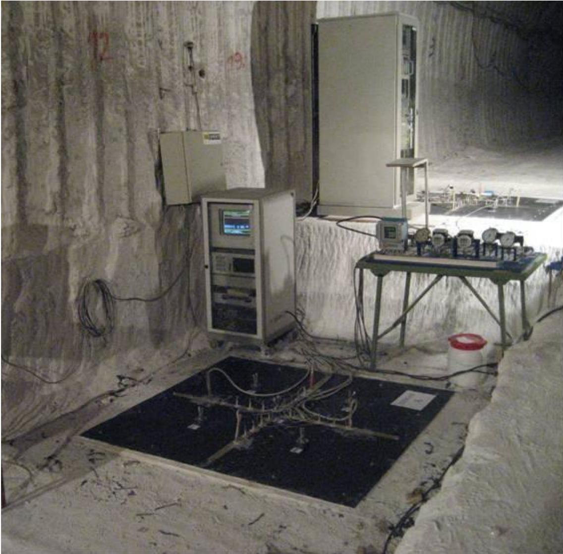
**Fig. 3-4** Test sites A (front) and B (back) with the 1-m cut-off (site A) and the brine injection and data collection systems
