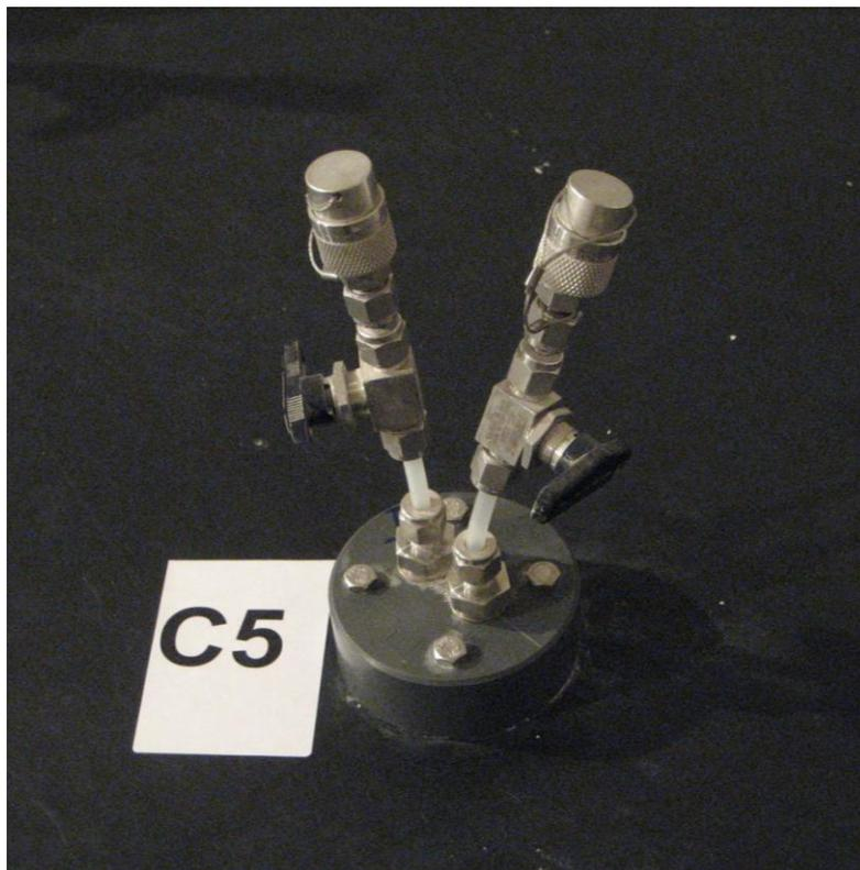
**Fig. 3-7** Borehole head with the tubes, valves and quick connectors for gas and brine injection or extraction
