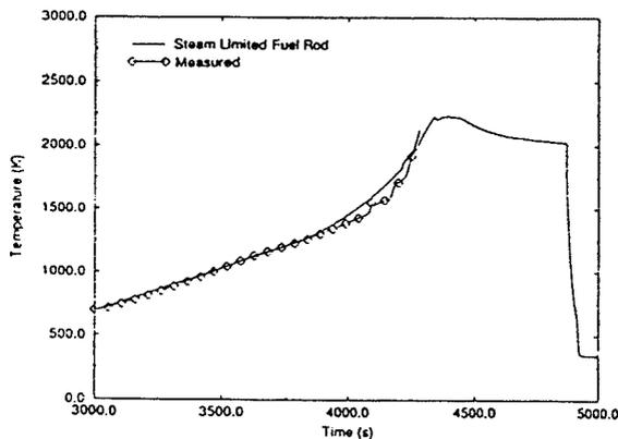
Figure 6. Calculated and measured temperatures at the 550 mm elevation when reflood hot spots in the bundle are modeled using a  $ZrO_2$  failure temperature of 2250 K.
