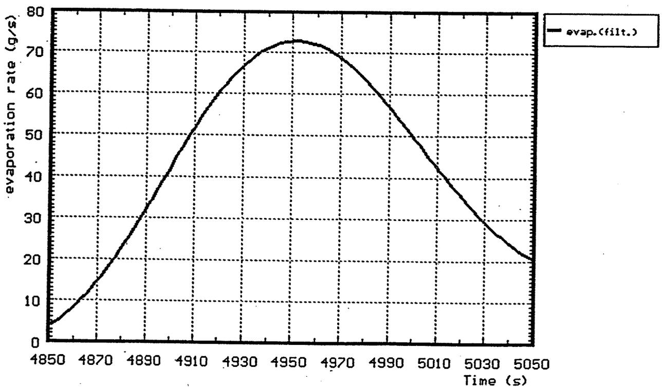
**Fig. 3.14:** Epavoration rate (g/s) during the quench process
