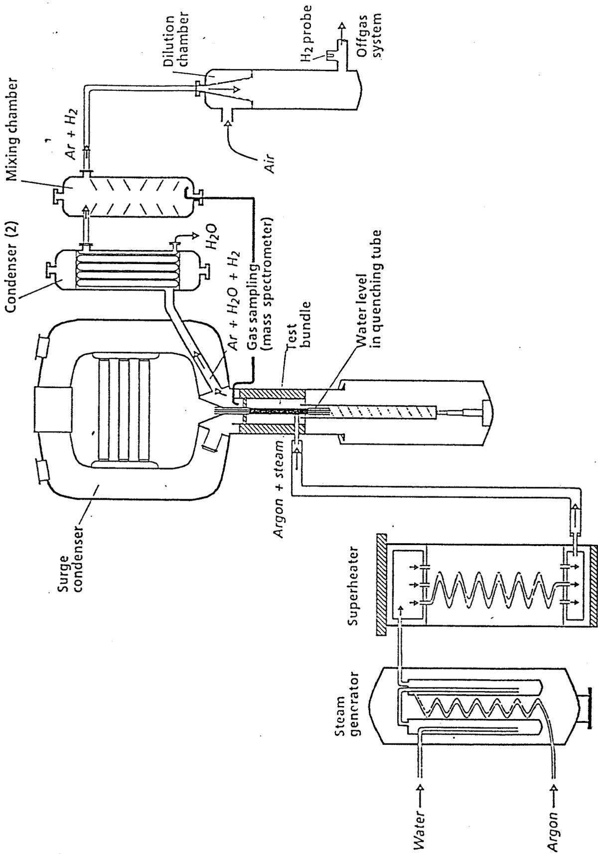
**Fig. 3.1: SFD Test Facility (Simplified flow diagram)**
