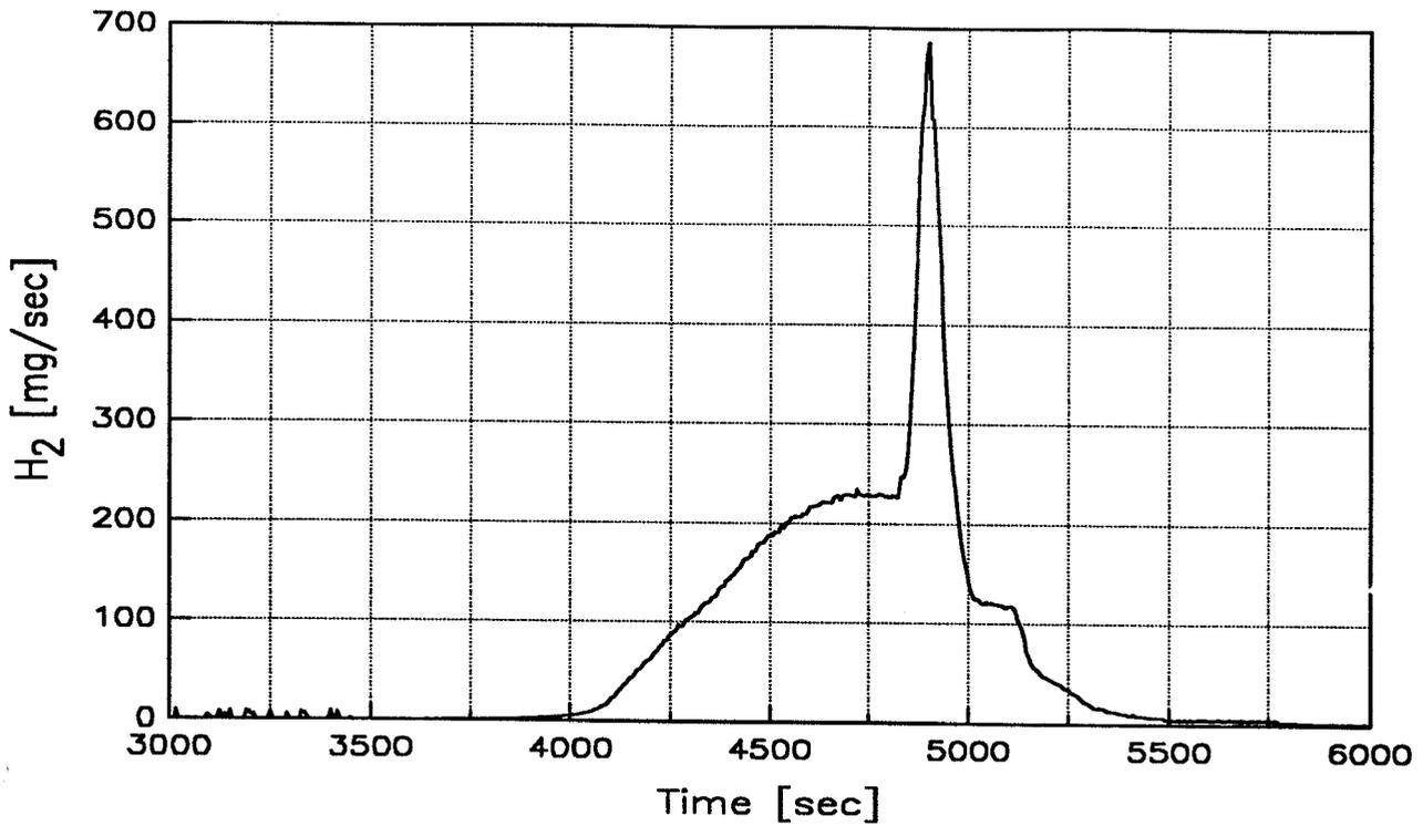
Fig. 3.19: Hydrogen generation during Test CORA-13 as measured
