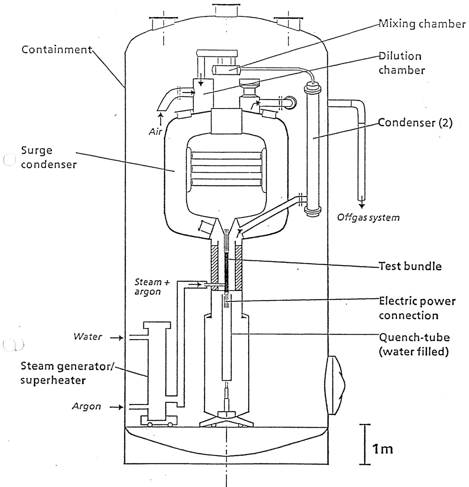
**Fig. 3.2: SFD Test Facility (Main components)**
