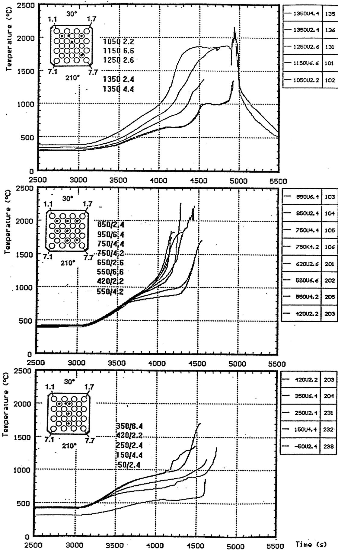
Fig. 3.15: Temperatures of the unheated rods (CORA-13)
