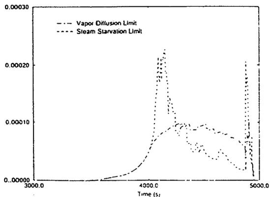
Figure 5. Hydrogen production rates from the steam starved and vapor diffusion limited cases.
