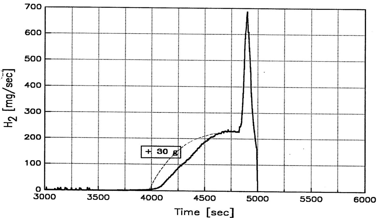
Fig. 3.19a: Hydrogen generation during Test CORA-13 Best estimate after adding of distributed hydrogen
