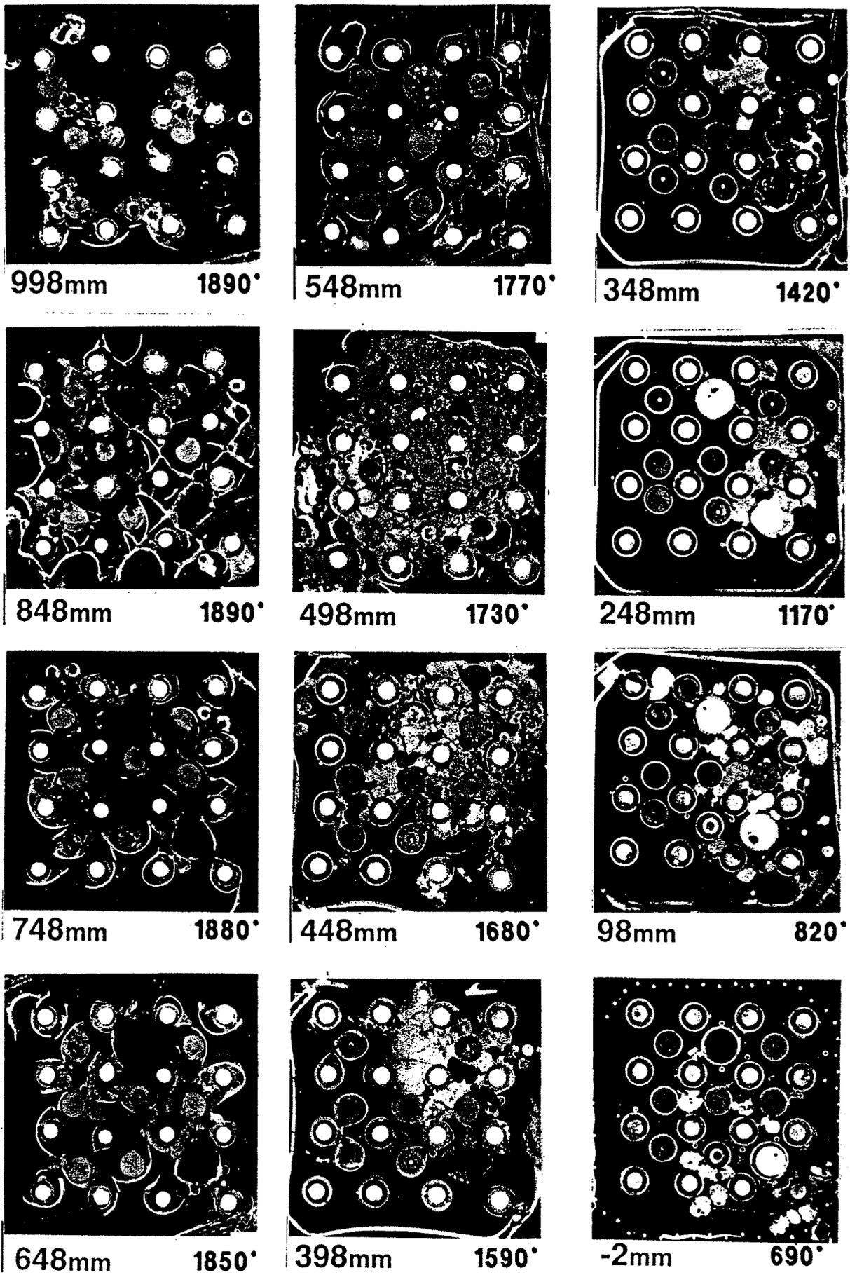
Fig. 3.21: Horizontal cross sections of bundle CORA-13
