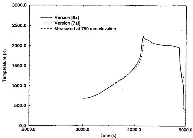
Figure 1. Comparison of calculated fuel rod temperatures from Version [7af] and [8x] with measured at 750 mm elevation.
