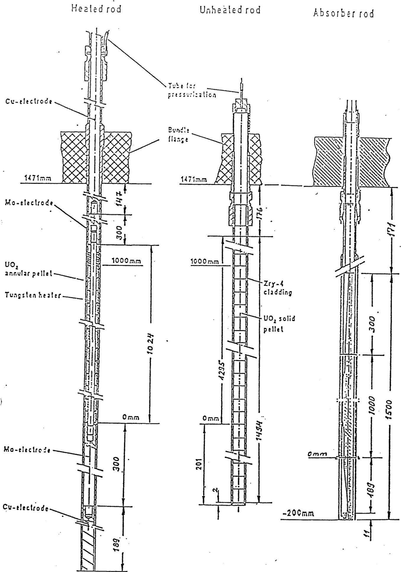
Fig. 3.6: Rod types used in the CORA experiments
