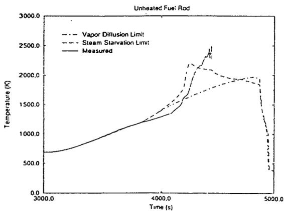
Figure 3. Calculated and measured temperatures at the 550 mm elevation - vapor diffusion and steam starved limitations.
