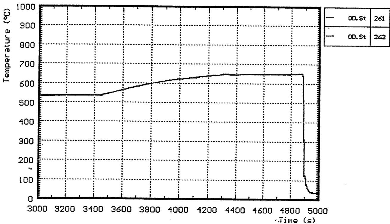
**Fig. 3.8: Temperatures at steam inlet (CORA-13)**
