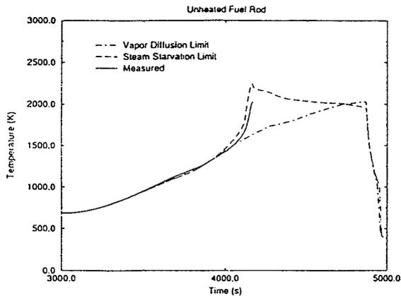
Figure 4. Calculated and measured temperatures at the 750 mm elevation - vapor diffusion and steam starved limitations.
