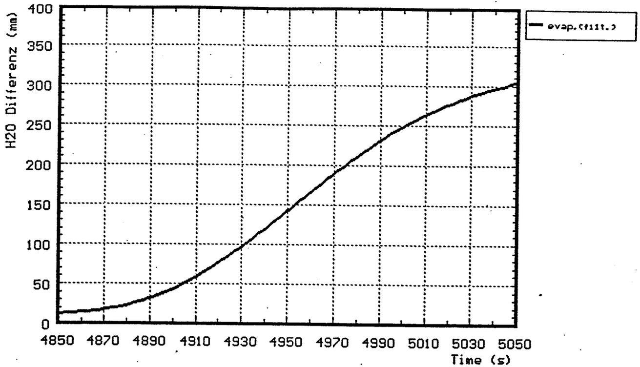
**Fig. 3.13:** Epavorated water from quench cylinder during the quench process (corrected for additional water input) (CORA-13)
