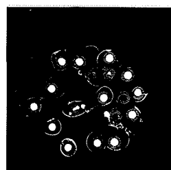
Fig. 3.16 Horizontal cross sections of bundle CORA-W2
