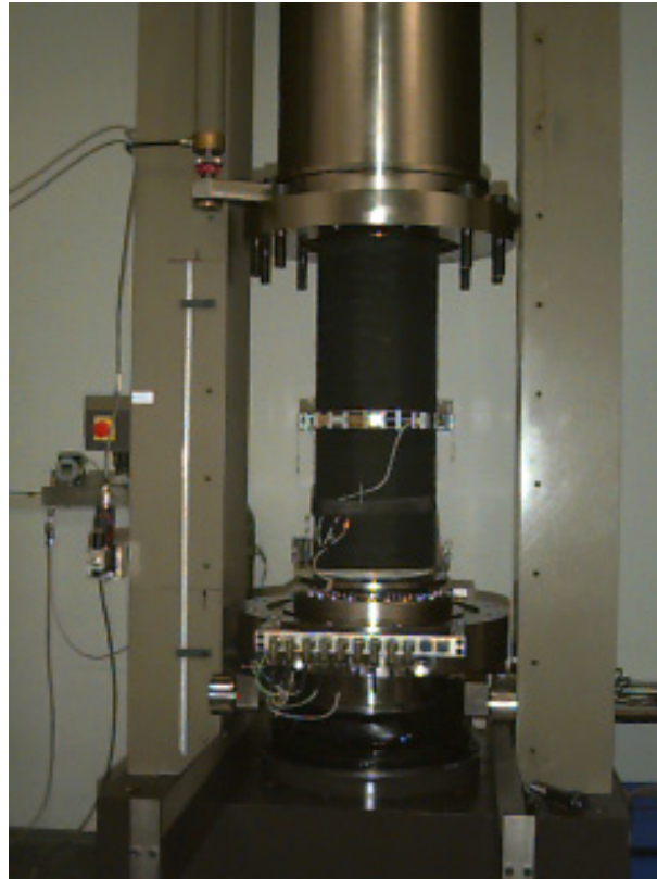
Figure 3-4 MTS triaxial test machine with inserted jacketed cylindrical crushed salt sample, the vessel is uplifted. In the mid-height of the sample a device for diameter measuring is shown.
