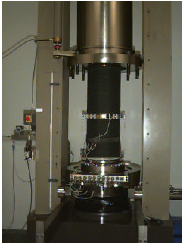
Fig. 7.10 MTS large triaxial cell with inserted jacketed cylindrical crushed salt sample; the vessel is uplifted. In the mid-height of the sample, a device for the measurement of the sample diameter is shown
