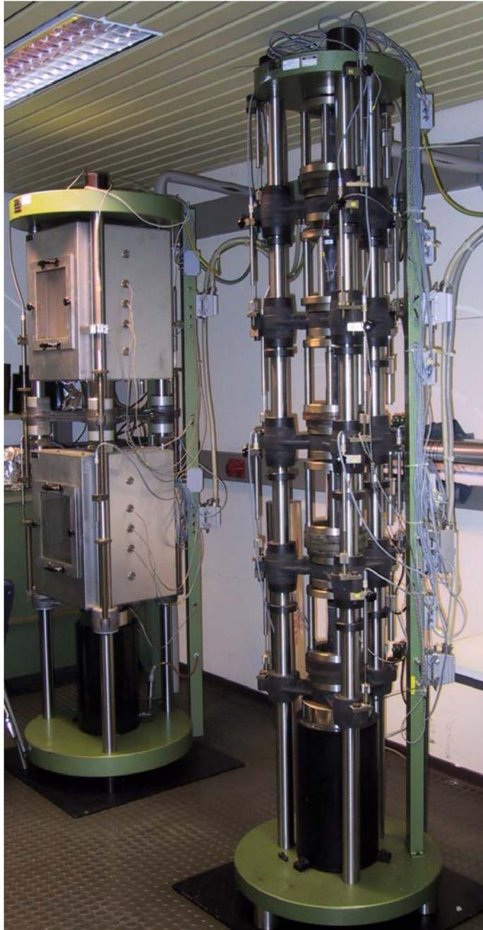
**Figure 5-1** Uniaxial testing machines for two and five simultaneous creep tests at GRS geotechnical laboratory in Braunschweig
