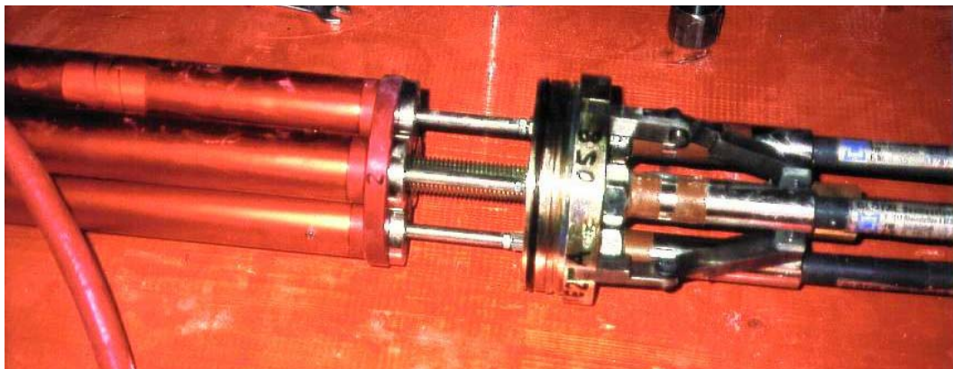
Fig. 5.3.12 Open instrument head of extensometer type Glötzl TEX 16 holding the electric displacement transducers (left side) with already connected extensometer protection tubes holding the glass fibre rods (right side)
