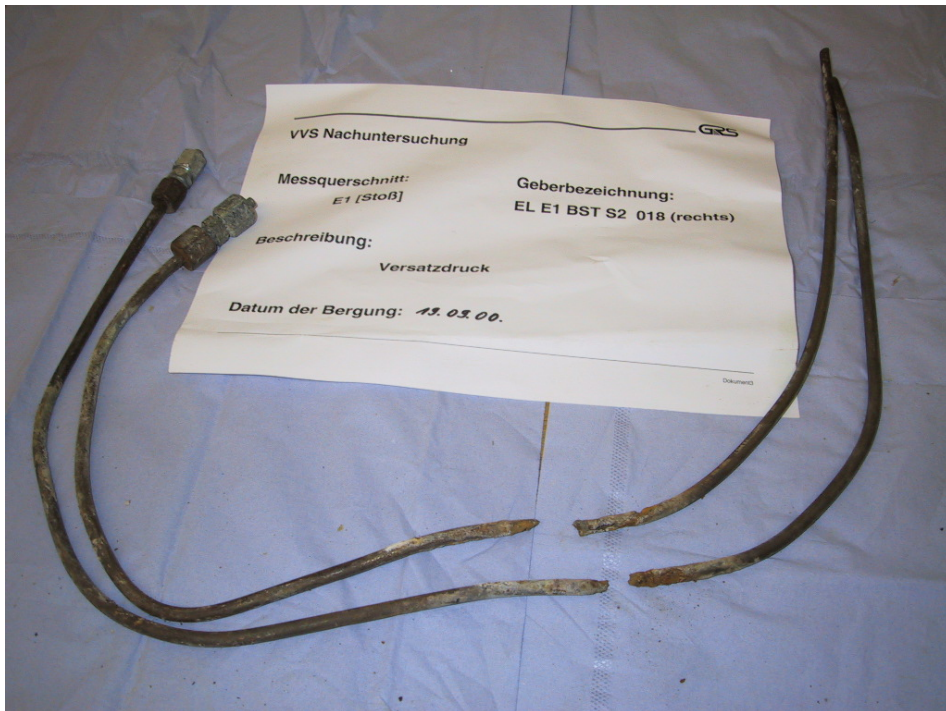
Fig. 5.4.2 Corroded hydraulic measuring lines of pressure gauge 61975
