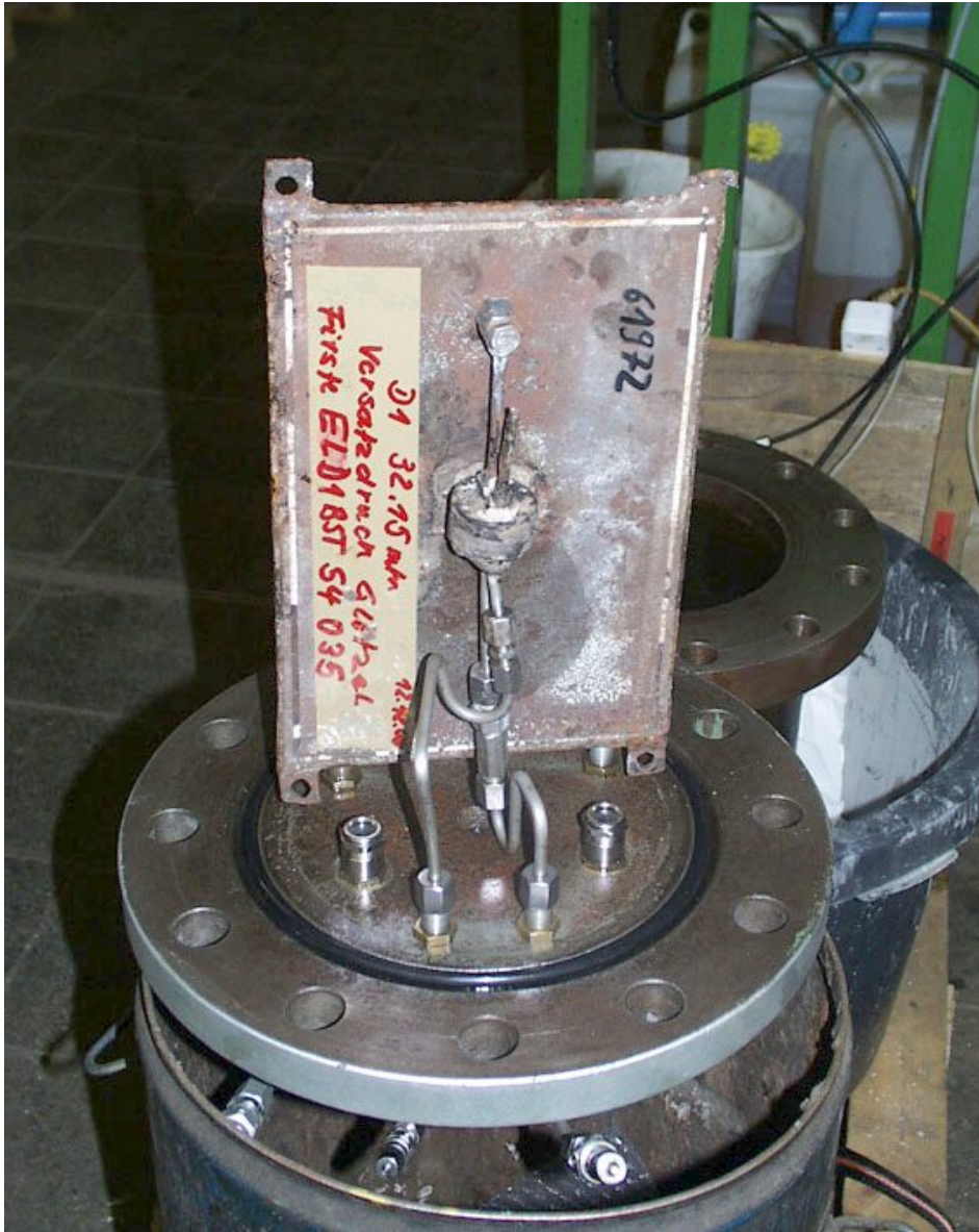
Fig. 5.4.7 Pressure gauge 61972 before calibration in the autoclave
