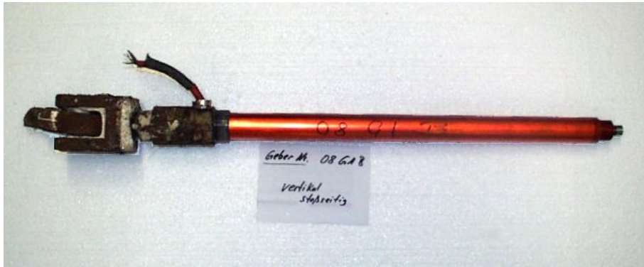
Fig. 5.3.3 Electric displacement transducer type Glötzl GWD 35/400 (sensor 8) after dismantling (spherical joint of the protection tube still mounted)
