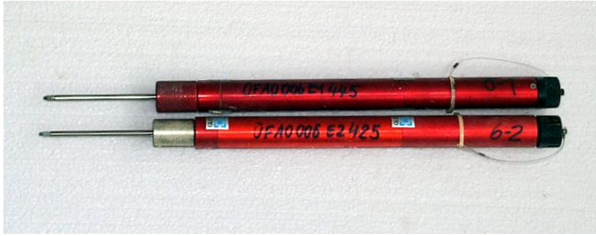
Fig. 5.3.14 Electric displacement transducers type GWW 50/50 (borehole 006: sensors 1 and 2)
