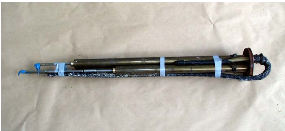
Fig. 5.3.8 Electric displacement transducers type Glötzl GWD 35/400 (sensors 16 and 17) and GWD 35/250 (sensor 18) after dismantling (lid of the instrument head still mounted)
