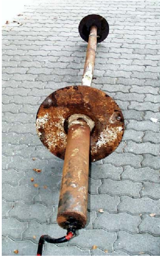
Fig. 5.3.7 Backfill settling measuring device from cross section B +1 : Instrument head (foreground) and two anchor plates with part of the protection tube between
