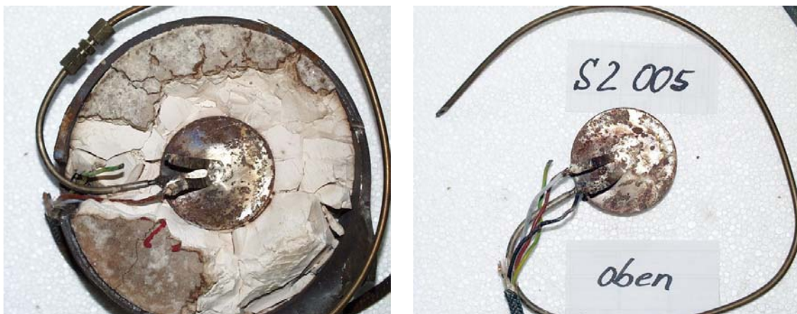
Fig. 5.4.11 AWID gauge 257 with pneumatic and electric measuring lines. a: During removal of its saltcrete embedding. b: After retrieval.
