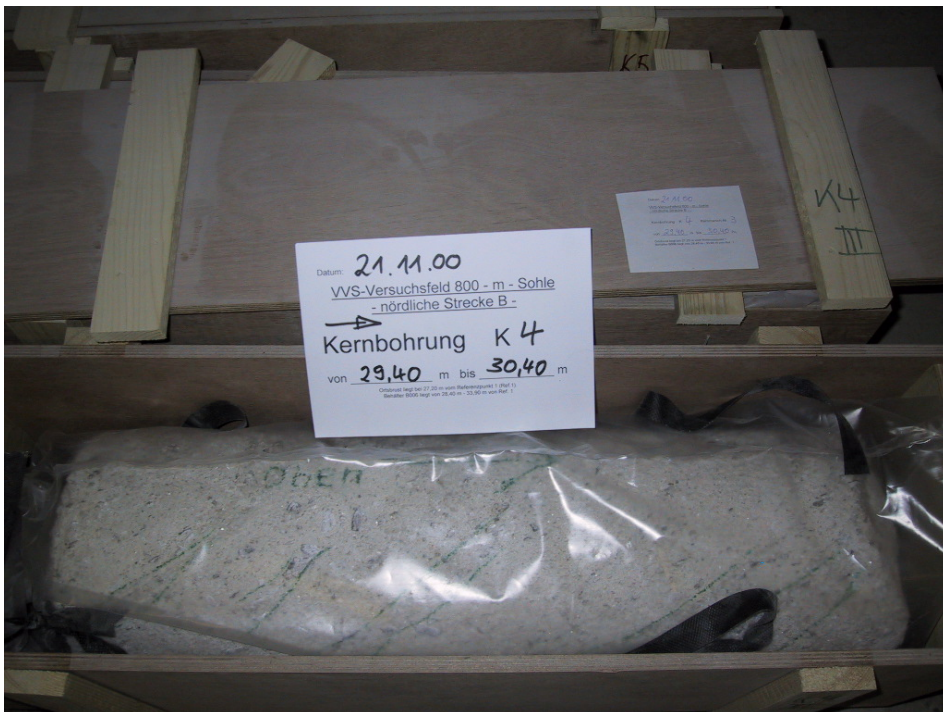
Fig. 3.8 280-mm core ready for shipment to the laboratory
