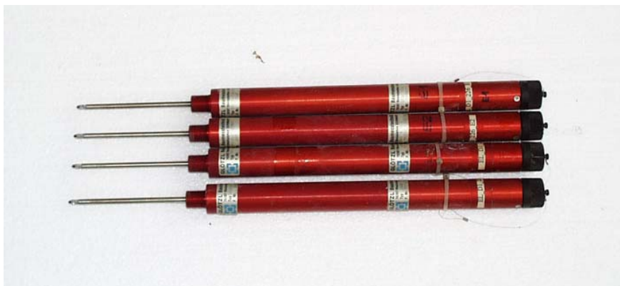
Fig. 5.3.16 Electric displacement transducers type GWW 100 I (borehole 226: sensors 37 to 40)
