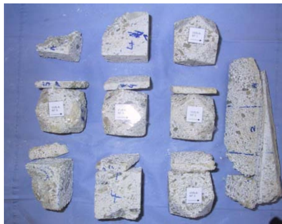
Fig. 4.4.2 Sample VVS-A-MI8. a: Identification of specimens. b: Prepared cubes for neutron texture analysis and slices for thin sections
