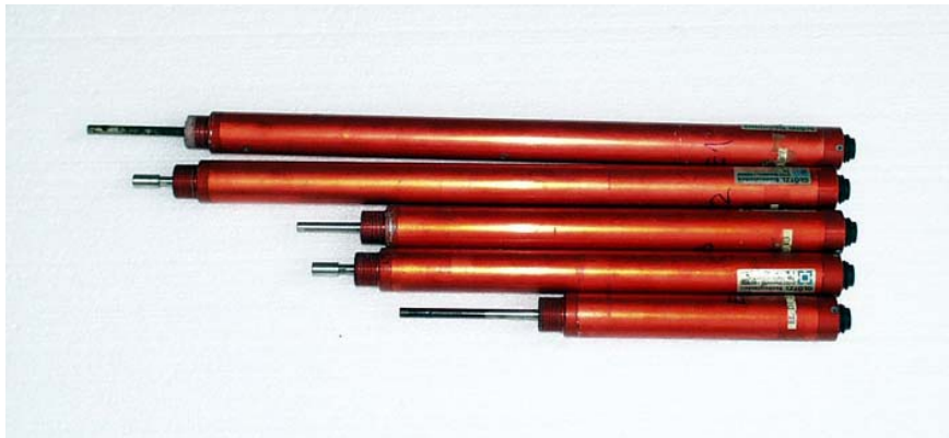
Fig. 5.3.15 Electric displacement transducers type GWD 35/400 (borehole 225: sensors 33 and 34), GWD 35/250 (borehole 225: sensors 35 and 36), and GWD 35/100 (borehole 225: sensor 14)
