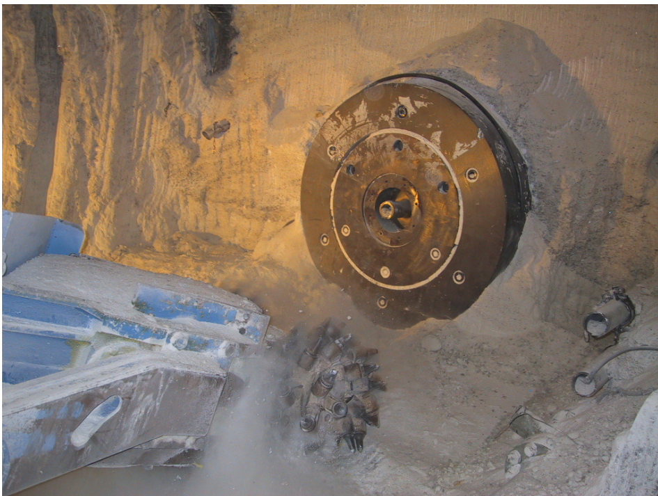
Fig. 3.2 Backfill excavation in the heated area using a continuous miner
