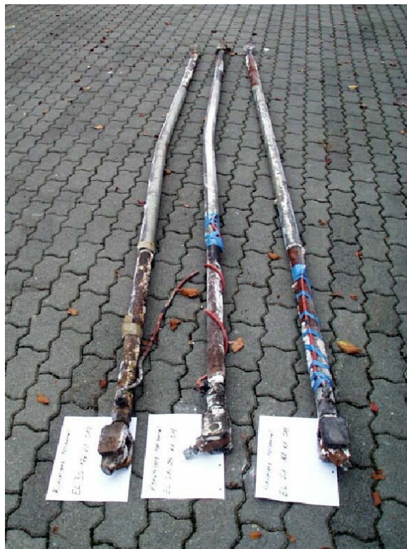
Fig. 5.3.2 Horizontal convergence measuring devices from cross sections B +1 and D1 -1 (both bent) and G1 (not bent) showing different corrosion of the protection tubes
