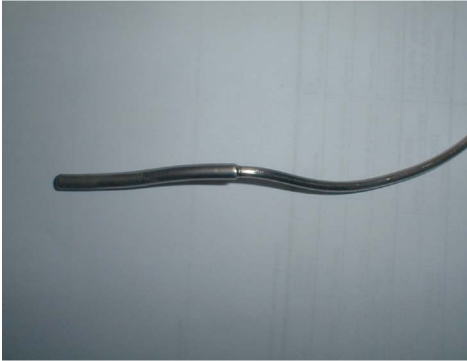
Fig. 5.2.5 Damaged temperature sensor from cross section F1
