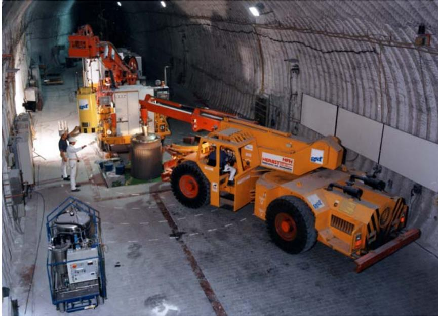
**Figure 6.1** Testing of a HLW disposal system/concept in the Asse mine/URL.
