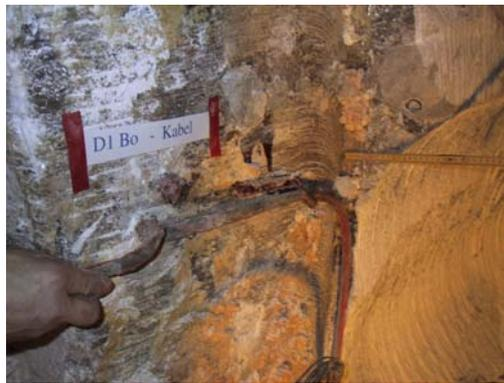
**Figure 3.11b** Squeezed cable in a cable slot in the drift wall at cross section D1 of the TSDE test field
