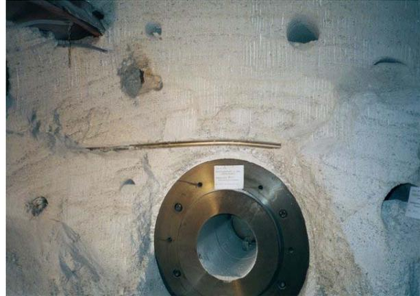
**Figure 3.10** Bent convergence measuring device
