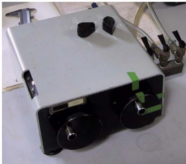
**Figure 5-3** Air comparison pycnometer (after Beckman)
