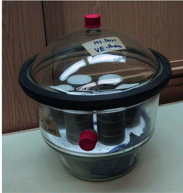
**Figure 5-2** Exsiccator with clay samples
