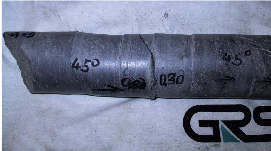
**Figure 7-10** Two core samples taken from the inclined borehole BVE 88 (depth: 0.15 m - 0.3 m and 0.3 m - 0.44 m)
