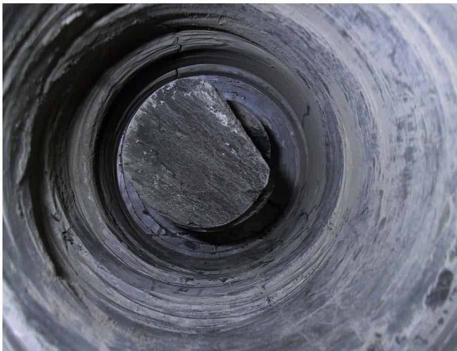
**Figure 7-9** View into a borehole before removal of the core sample
