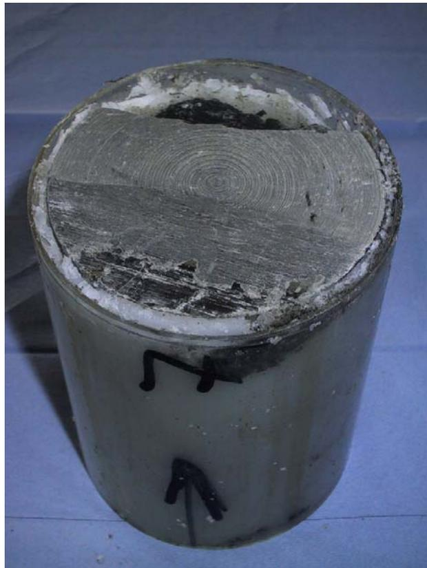
**Figure 5-1** BVE sample poured with wax in a plastic tube
