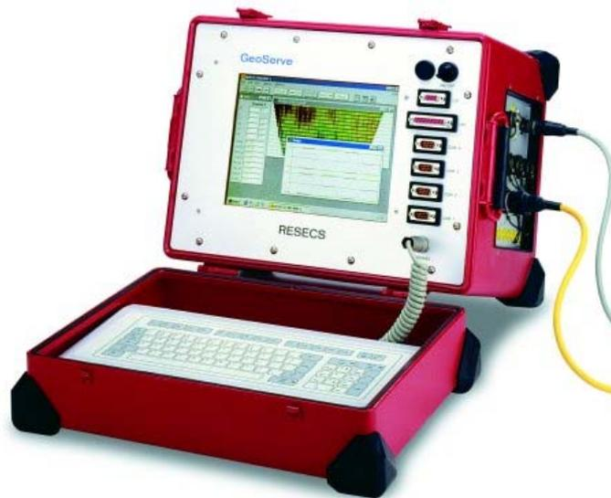
**Figure 3-1** RESECS measuring system
