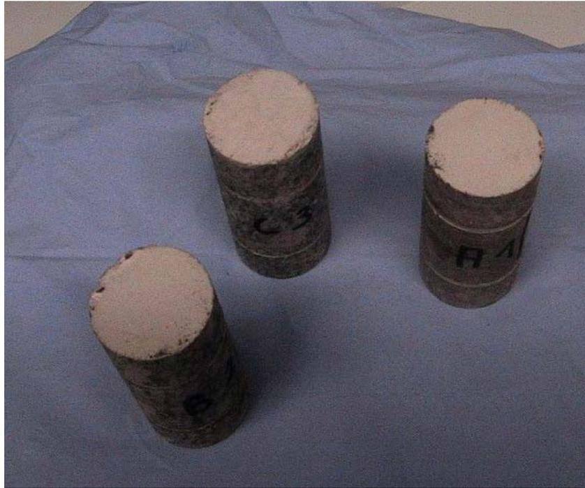
**Figure 5-10** Sample coated with conductivity silver lacquer
