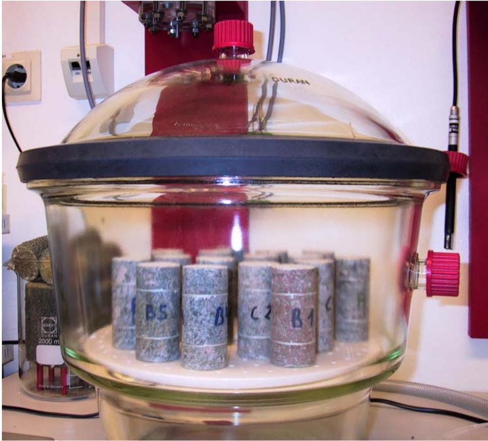
**Figure 5-7** Exsiccator with granite rock samples
