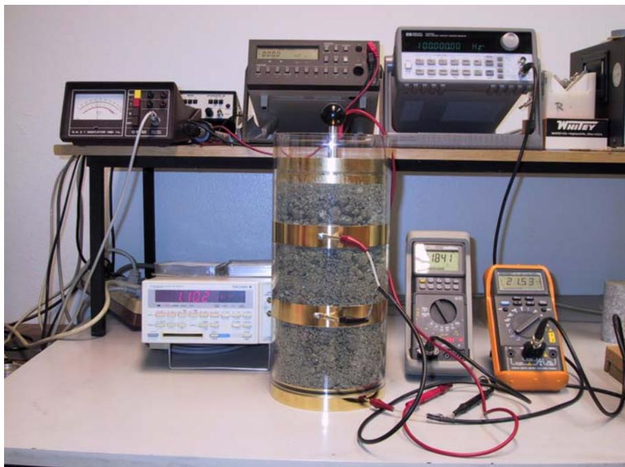
**Figure 5-5** Measurement set-up for determination of backfill resistivity
