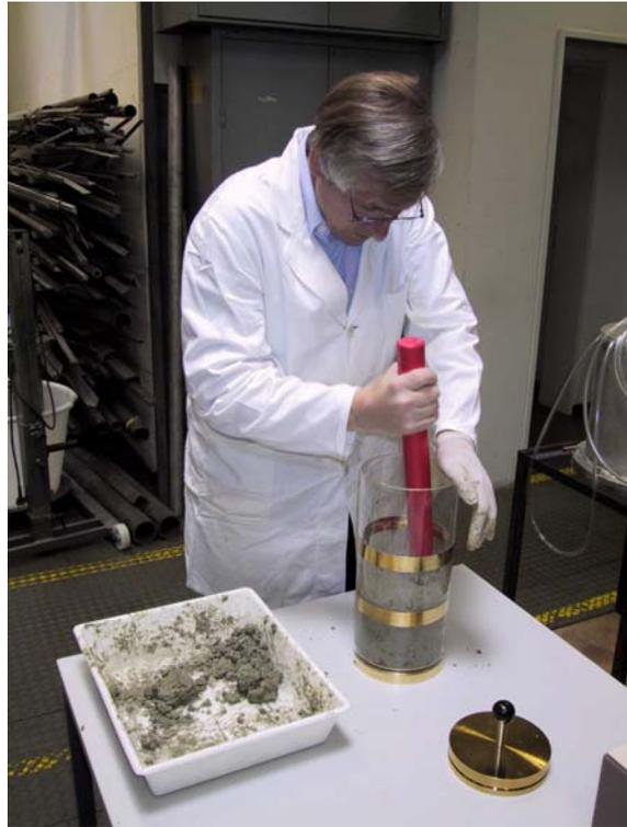
**Figure 5-4** Emplacement of moistured backfill into measurement cell for determination of material resistivity
