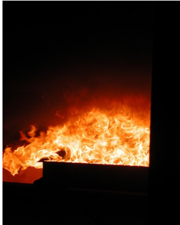
Fig. 3-1 Fire development inside the fire compartment - Test 1, view through front door
