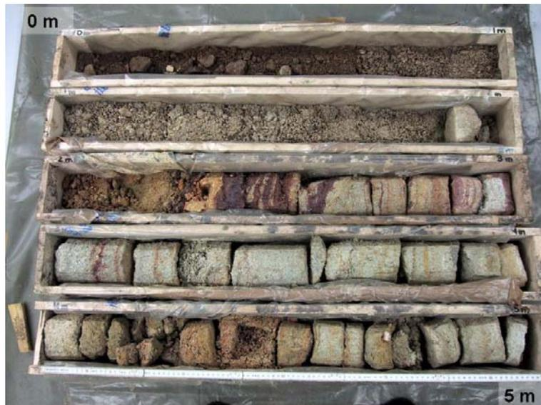
**Fig. 7:** Drilling HB08-02: Cover (0 - 2.5 m); Burgsandstein below 2.5 m
