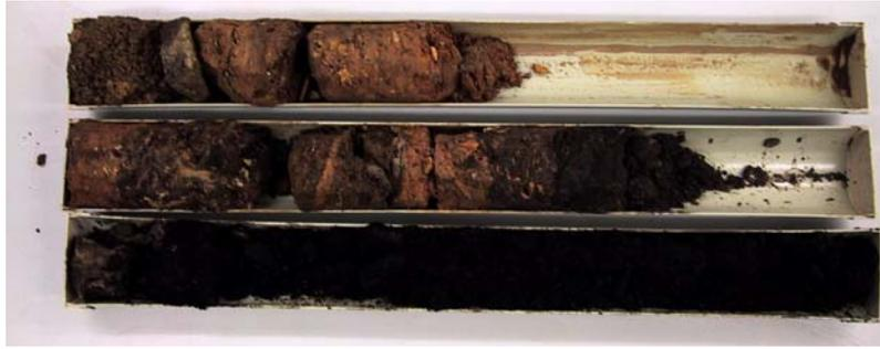
**Fig. 14:** Example of drill core storage in PVC tubes (HB05-02 0 - 3 m)
