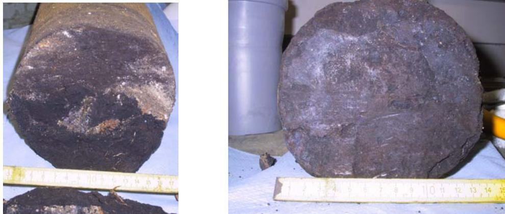
**Fig. 22:** Samples used for permeability measurement. Drill core HB11-03/1,00 – 1,035
