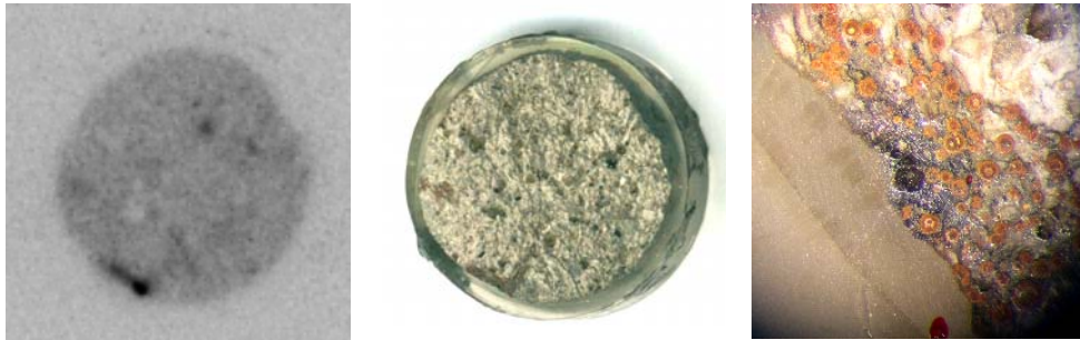
Fig. 5.14: Image of the borecore sample NA4 34,5 m (middle) autoradiographic image (left) and optical microscopic 2.1 mm x 2.1 mm image of the lower left area with hot spot (pyrite nodules appear orange, lignite black and clay white)
