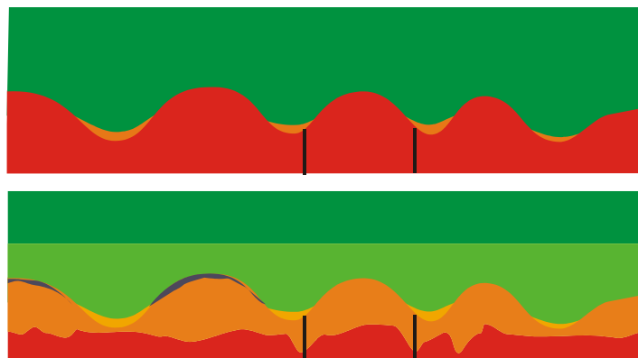
Fig. 6.2: Hypothesis A: Alteration of granite (red) to kaolin (orange) after deposition of volcanic ash (green).
