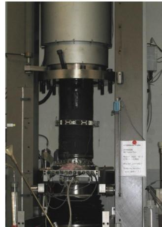
Sample embedded in rubber jacket in the MTS test apparatus.
