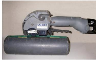
Sample installed in PVC tube with clamping device for axial clamping.
