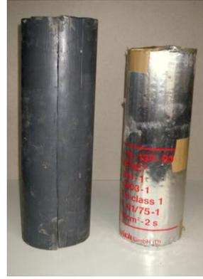
Sample supplied with aluminium coated plastic wrap and slitted PVC tube.
