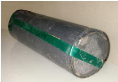
Axially clamped sample.
