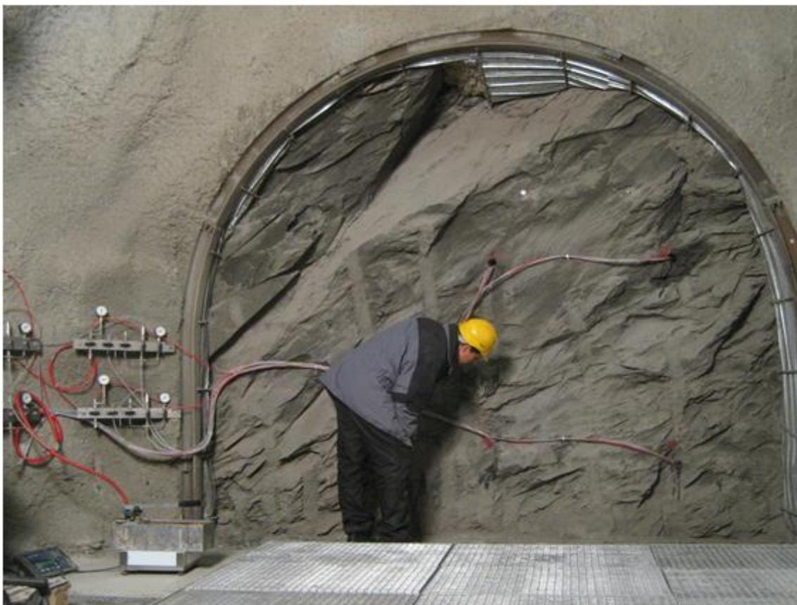
**Fig. 4.8** Borehole collars of BMB 1 – BMB 4 and transducer racks (left)
