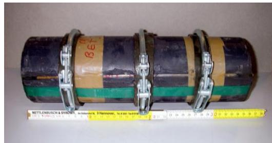
Radially clamped sample using clamping collar.
