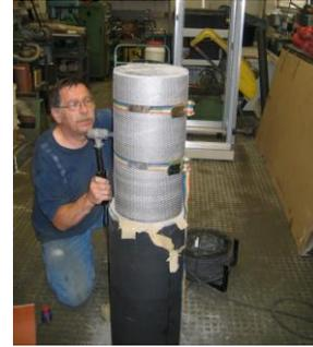
Covering the sample with a punched plate, soldering the seam of the plate.
