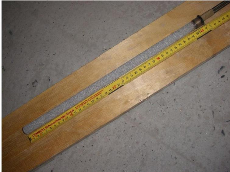
**Fig. 4.3** Minipiezometer installed in the test boreholes
