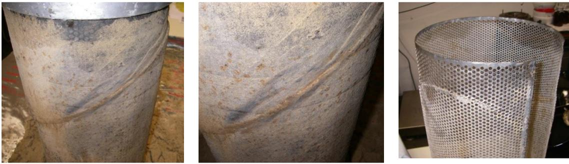
**Fig. 5.20** Removed sample 3L after the end of the test (left: healed shear plane, centre: zoomed in view, right: punched plate with shear mark)
