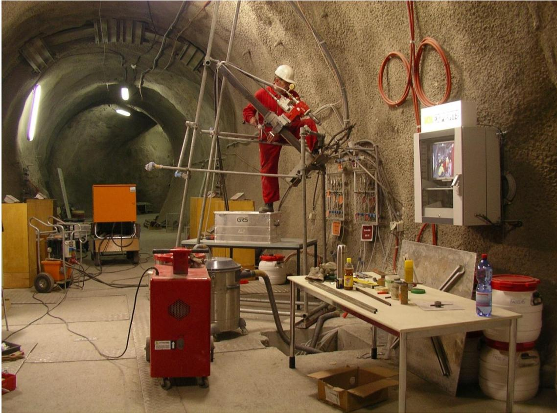
**Fig. 4.2** Drilling of test boreholes
