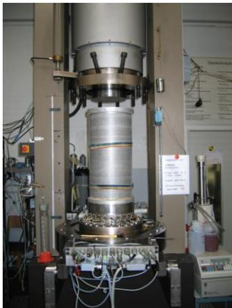
Installing the sample in the MTS test apparatus. Support straps were removed before complete installation.
