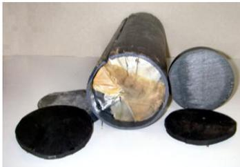
Sample installed in the PVC tube with rubber discs (front) and PVC stoppers (back) for the end planes.
