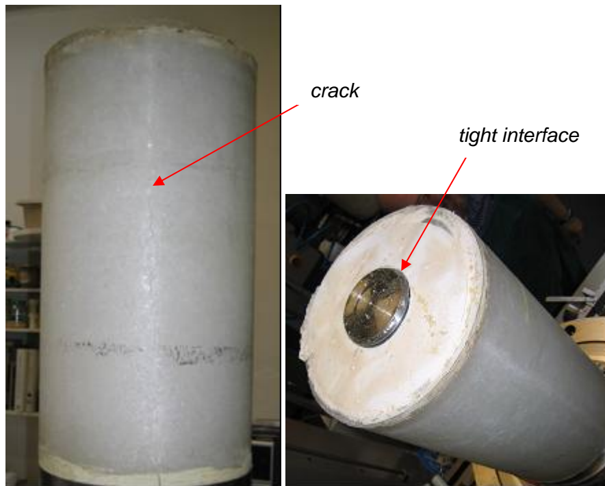
Fig. 3.15 Photos of the large hollow salt sample 1 after dismantling
