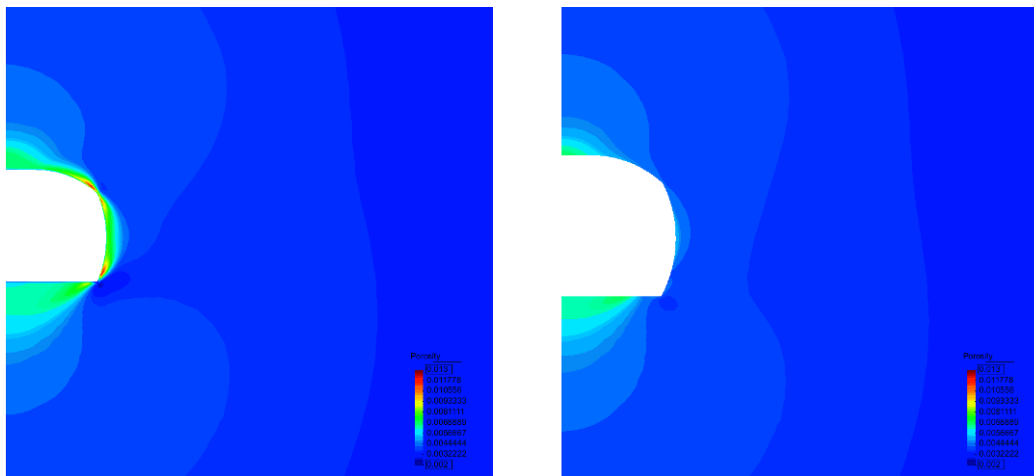
Fig. 6.4 Porosity around the drift before EDZ cut-off (left) and at the time of seal construction, six months after EDZ cut-off (right)
