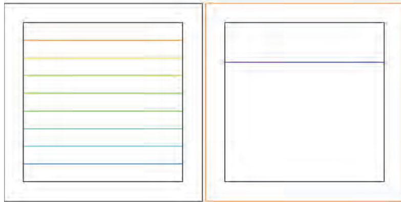
Fig. 6.2 Several contour lines (level sets) of the initial level set function (left) and zero contour line that defines the initial position of horizontal groundwater table (right)
