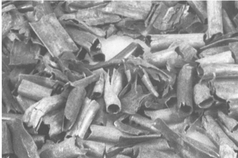
Fig. 1.3 Hulls from a fuel assembly irradiated in a pressurized water reactor in Obrigheim (Germany) after passing shearing and dissolution cells of the UP2 plant at La Hague /RES 92/
