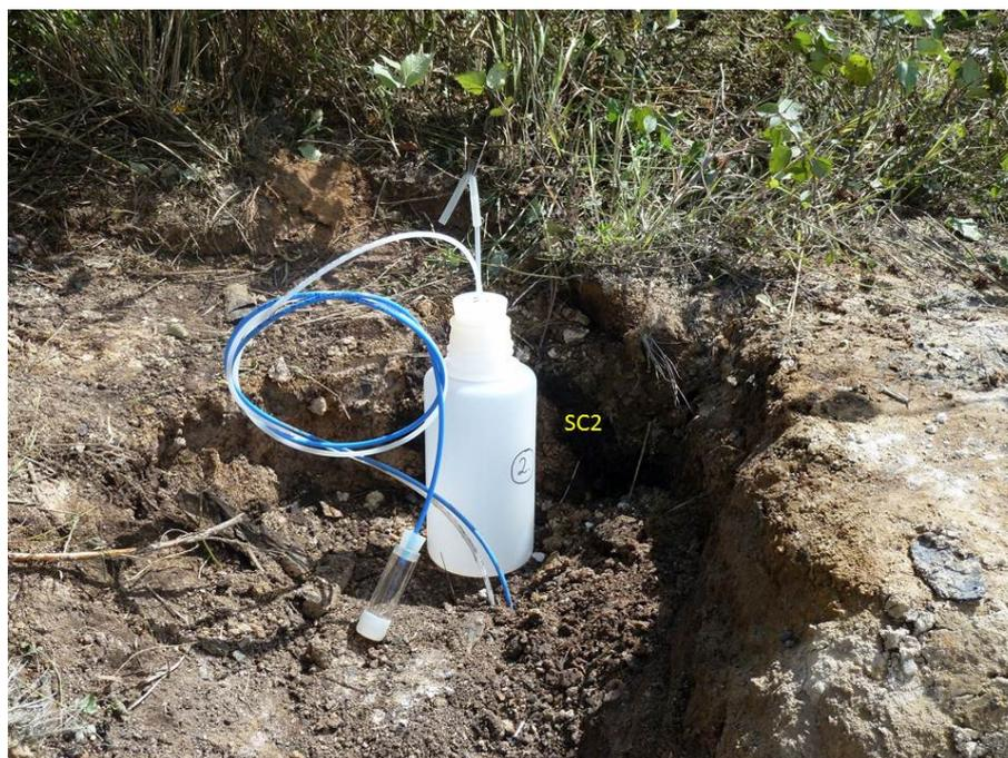
**Fig. 4.84** Position of installed suction cup 2 the cartridge is dug in at app. 100 cm depth
