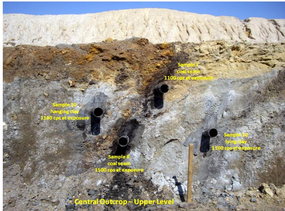
**Fig. 4.79** Coal seam in the upper level of open pit's outcrop at Ruprechtov site; results of gamma measurements as well as position of sampling is indicated
