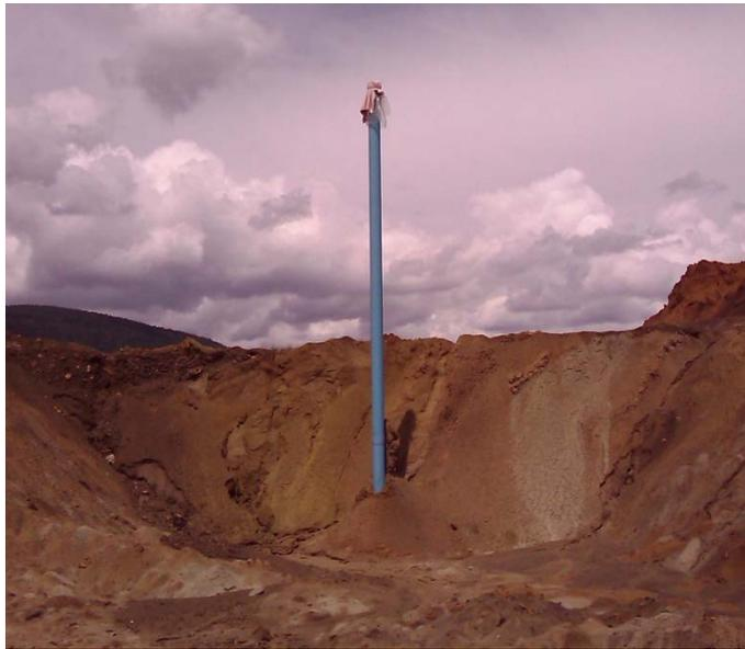
**Fig. 4.82** NAR3 drill hole after progress of mining activities in this area
