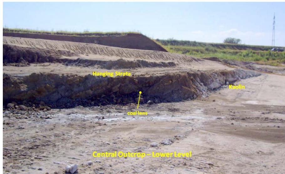
**Fig. 4.77** Central outcrop of kaolin open pit at Ruprechtov site showing inclined sediments of do-called hanging strata including coal lens on top of kaolin (right edge of the photograph)
