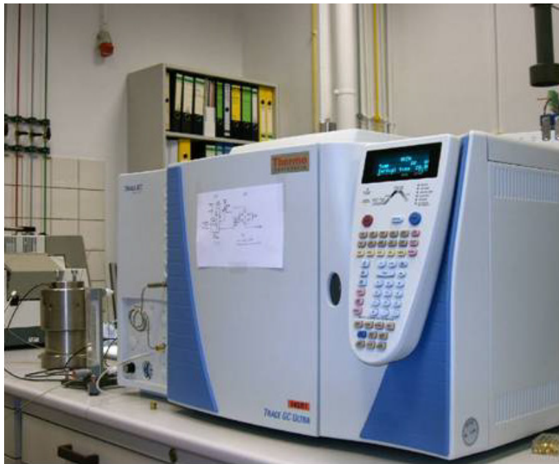
Fig. 5.1 Experimental setup for the investigation on diffusion in compacted MX-80 samples (left: diffusion cell; right: gaschromatograph)
