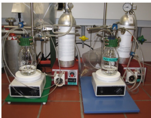
Fig. 4.1 Experimental set-up for the determination of gas dissolution
