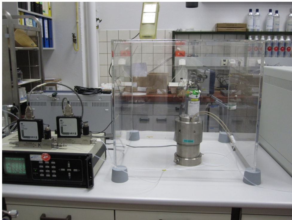
Left: Two mass-flow controller with data acquisition unit. Right: measuring device with an acrylic glass hood
