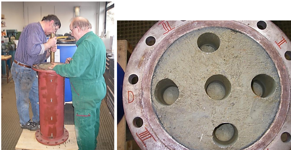
a) sampling with a core cutting tube b) sample locations at the upper end of the sand/bentonite seal
