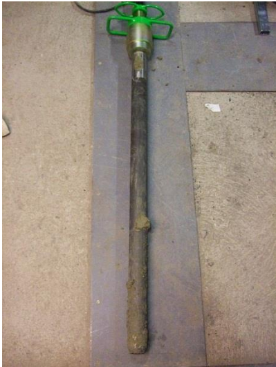
a) Filled driving rod
