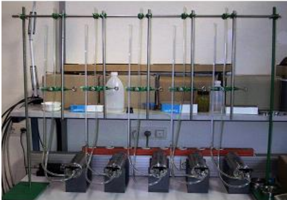
Fig. 2.3 Experimental set-up for saturation tests
