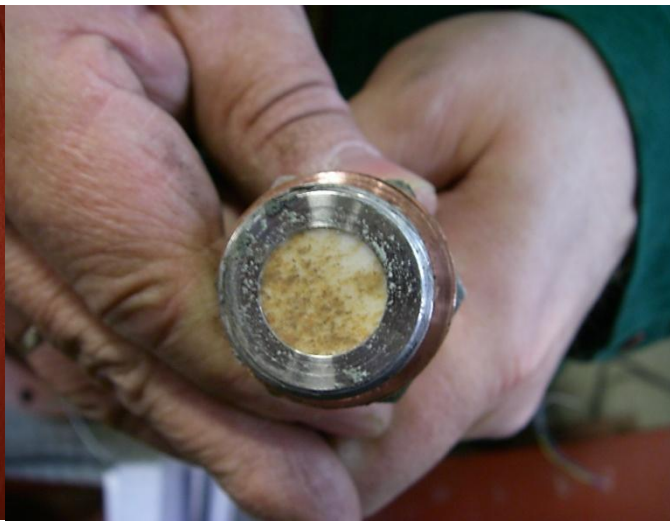
b) Dismantled swelling pressure sensor
