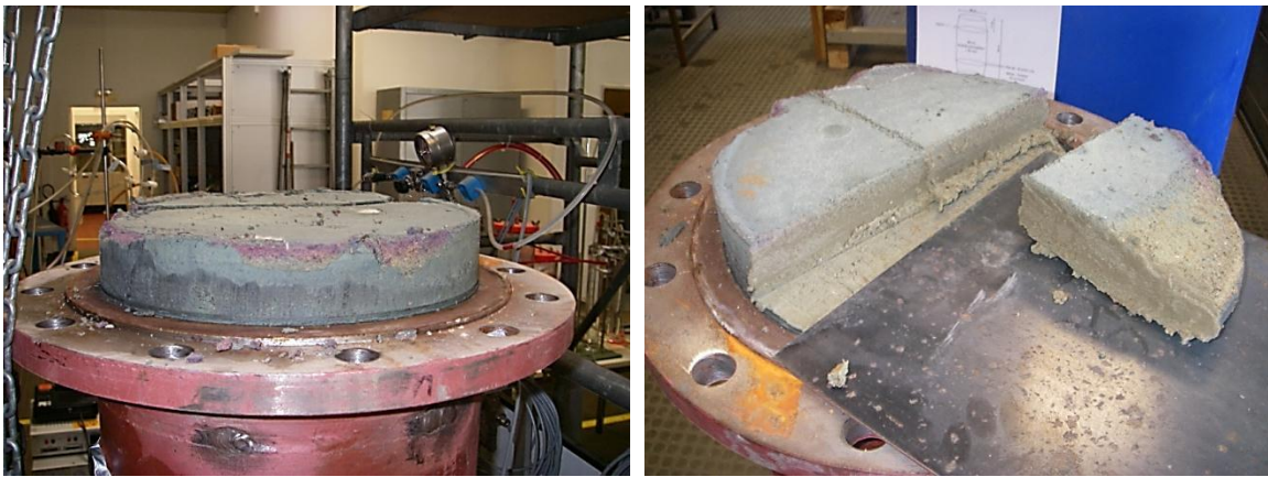
a) seal material emerging out of the mock-up test section
