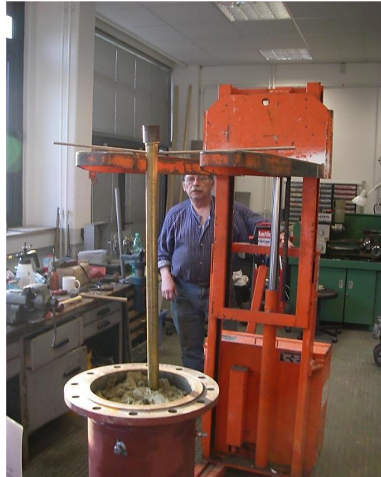
b) retrieval of the core cutting tube with a fork lift
