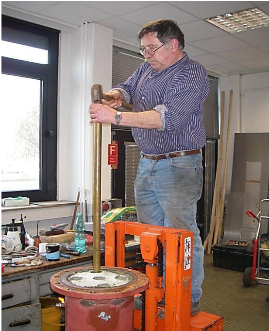
a) sampling by pushing a longer core cutting tube
