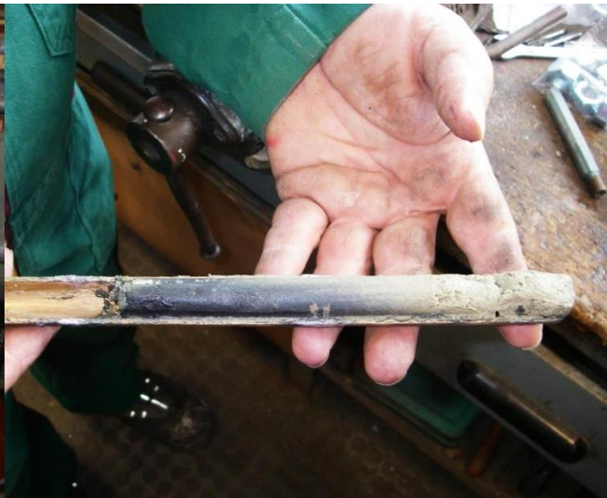
d) Uncovered sample taken horizontally from the mock-up test section
