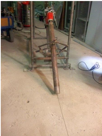
c) Drilling machine shortly before coring an inclined borehole
