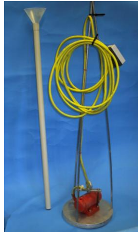
b) Electric vibrator and funnel
