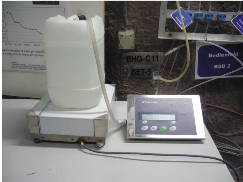
Fig. 5.17 Measuring container placed on a high precision balance located outside the borehole
