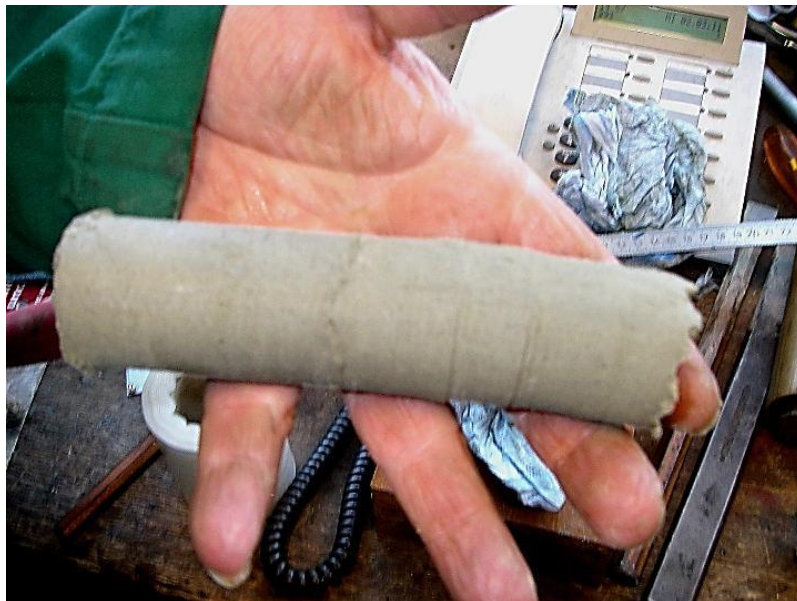
c) compacted seal material sample
