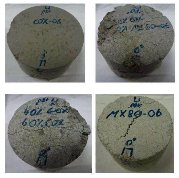
**Fig. F.54** Samples of the compacted claystone-bentonite mixtures after water saturation at RH = 96 % over 6 months
