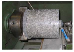
(a) Preparation of a cylinder of D = 250 mm / L = 243 mm from the compacted sample
