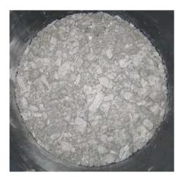
**Fig. 3.3** Photo of the crushed claystone with grains d < 32 mm after hand stamping
