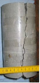
(a) COX sample (D/L = 100/200 mm) artificially-fractured
