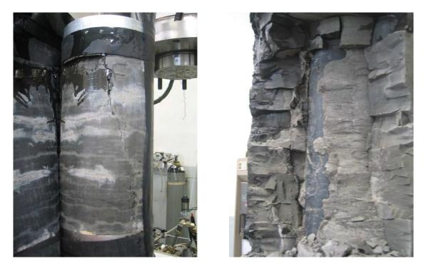
Fig. 2.79 Pictures of the large hollow cylinder EST45592 damaged after testing
