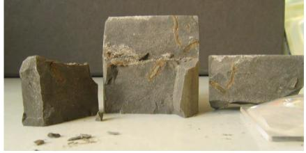
(e) COX sample EST27390A pre-confined after exposing to synthetic porewater
