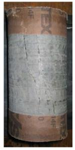
(b) OPA sample (*D*/*L* = 100/200 mm) naturally-fractured
