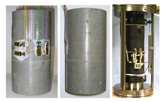
**Fig. 2.44** Pictures of a prepared COX sample and instrumentation for strain measurements during triaxial creep testing
