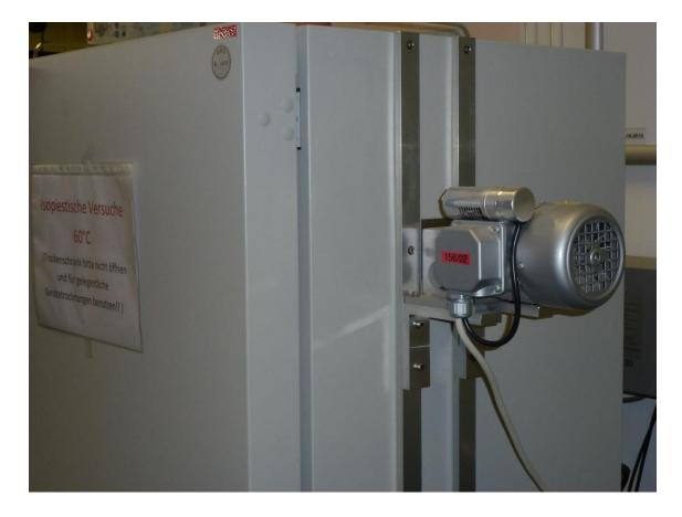
**Fig. 2.4** This picture shows a motor fixed at the outside of an oven to exert a gentle rocking motion to the board on which the isopiestic vessels rest
