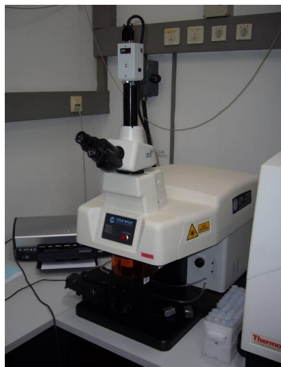
Abb. 5 Laser Ablations System „New Wave UP 213 Deep-UV YAG“ der Firma New Wave Research
