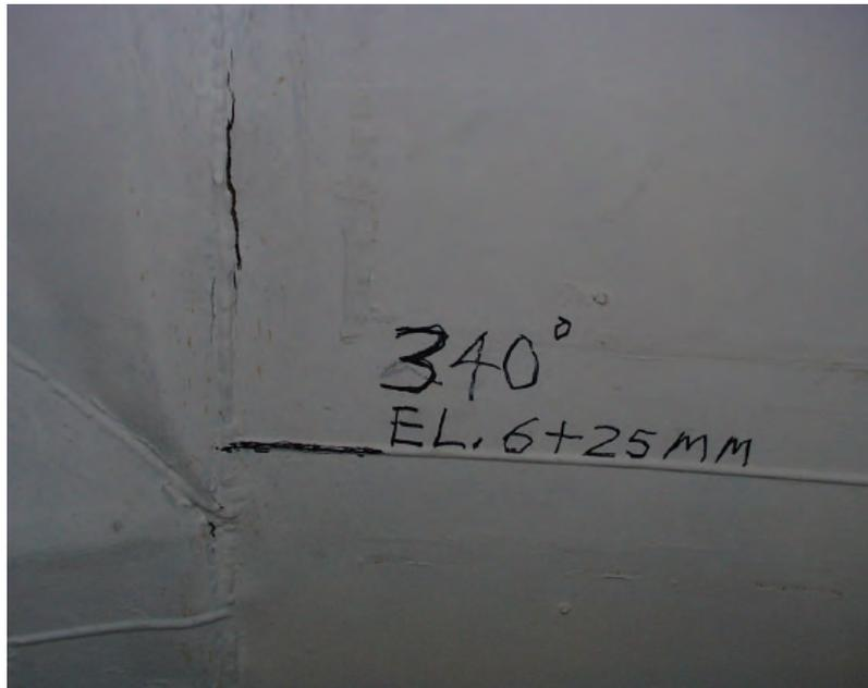
Fig. 12-10 Crack #15 in the liner localized at azimuth  $\sim 340^\circ$  (see Fig. 12-9) after the Limit-State-Test (LST) (from /SAN 03/)
