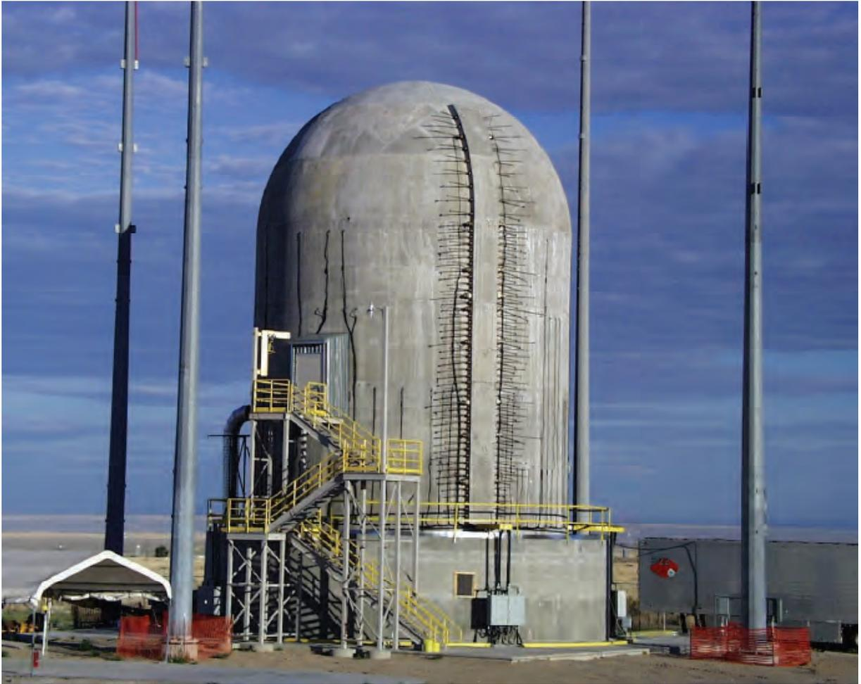
Fig. 12-8 Completed 1:4 scaled model of the PCCV (from /SAN 03/)
