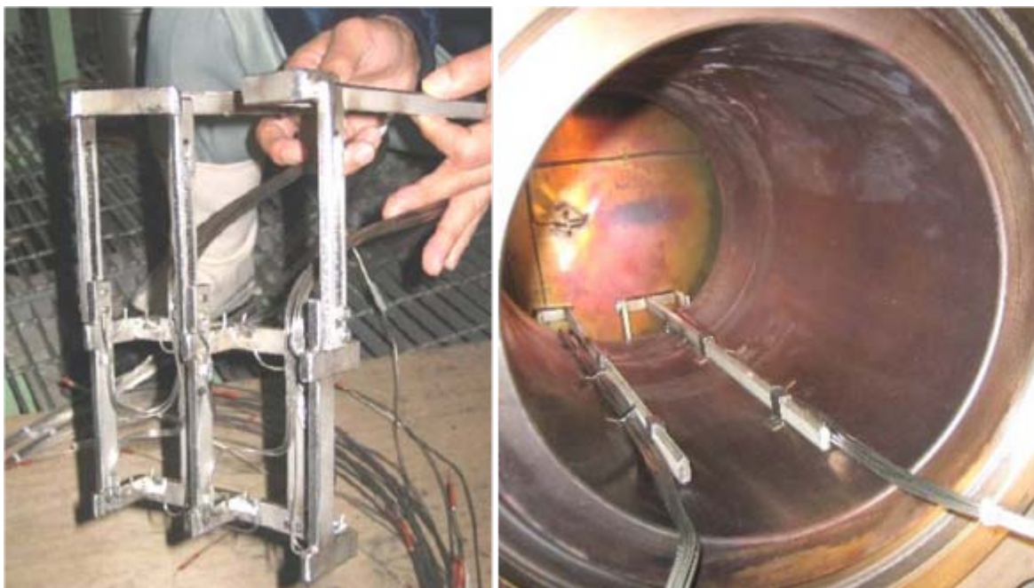
Figure 10: Frame structure of thermocouples of group TE4 and downcomer view from cold leg
