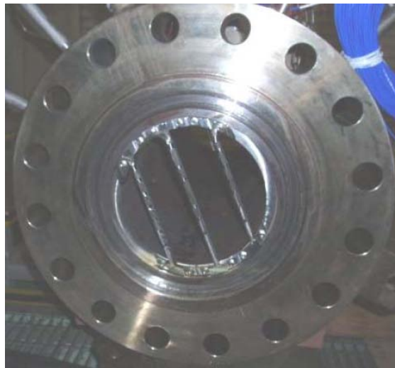
Figure 8: Thermocouples in spool piece flange
