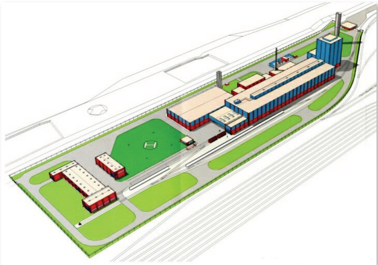
▲ Fig. 10: Planned surface facilities at shaft Konrad 2 for the future functions as the upcast ventilation shaft and the transportation shaft for the radioactive waste to be disposed of.
