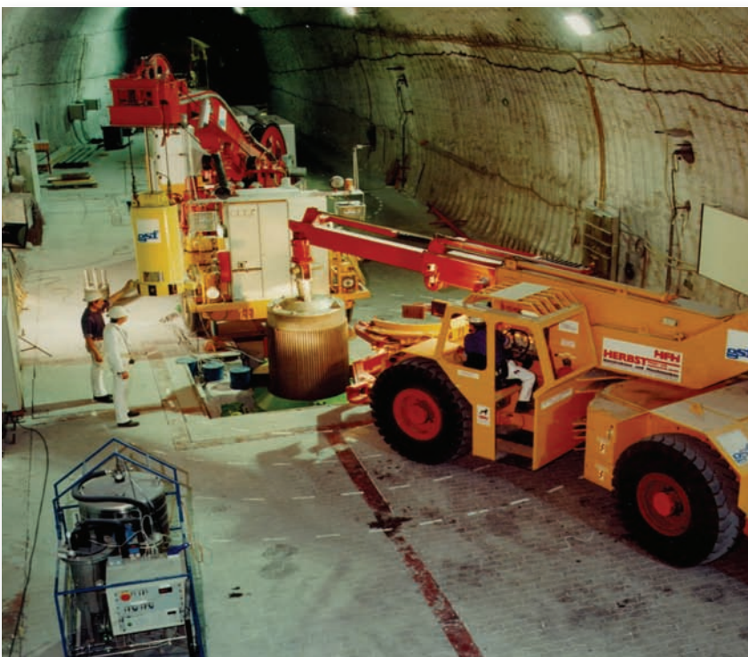
◀ Fig. 7: Demonstration of the disposal of high-active waste (test with empty drums)
