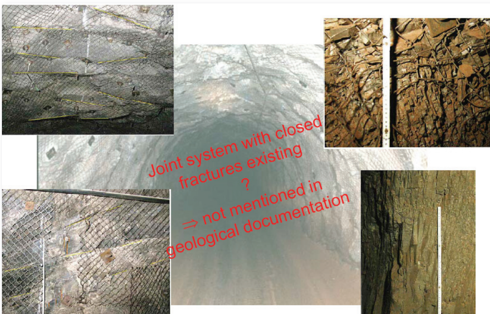
▲ Fig. 5: Additional detailed in situ investigations of rock mass structure and results
