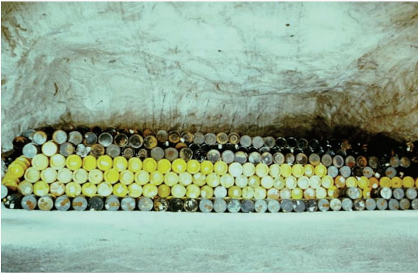
◀ Fig. 4: Disposal of low-active waste (horizontal stack)
