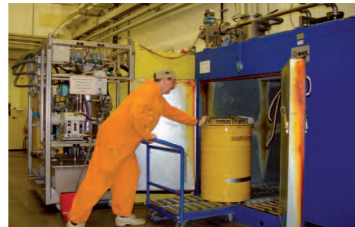
Fig. 39: Conditioning of waste (in-drum drying facility)
