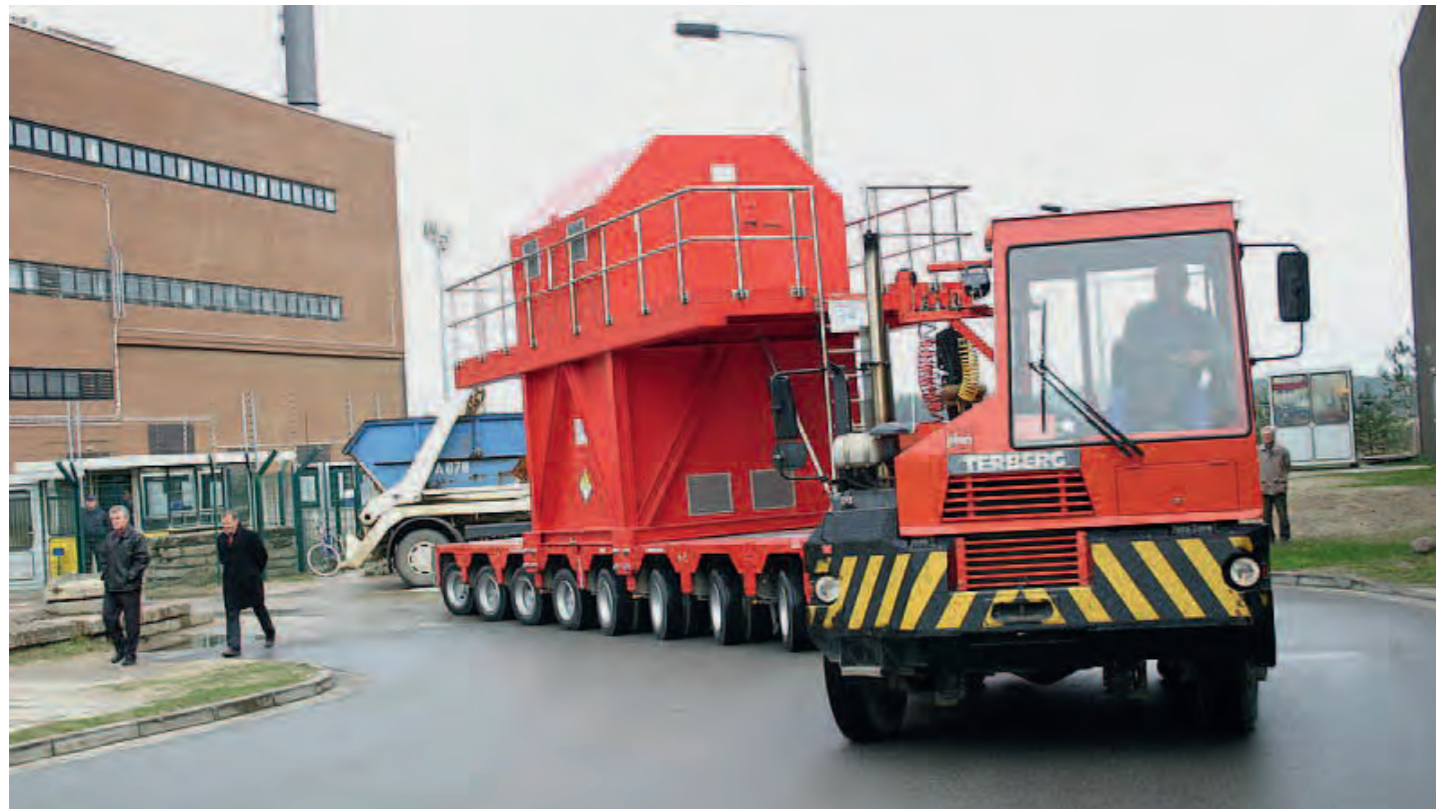
Fig. 21: Plant-internal transport of irradiated fuel assemblies
