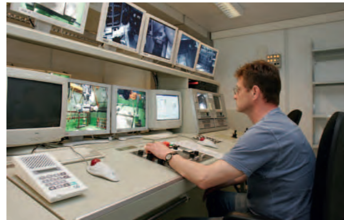
Fig. 29a: Remote-controlled thermal cutting (control room for remote-controlled work)
