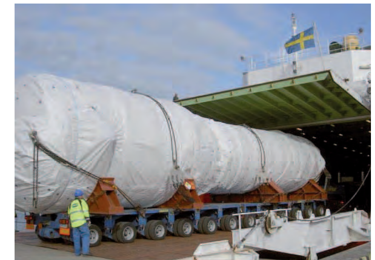
Fig. 30: Transport of a steam generator to Sweden for melt-down
