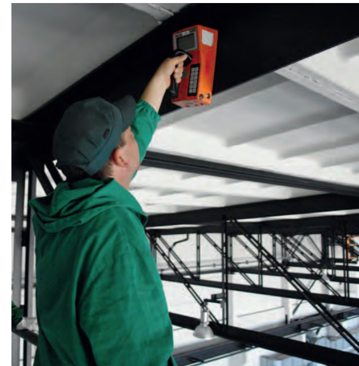
Fig. 16: Measurement to determine a possible contamination
