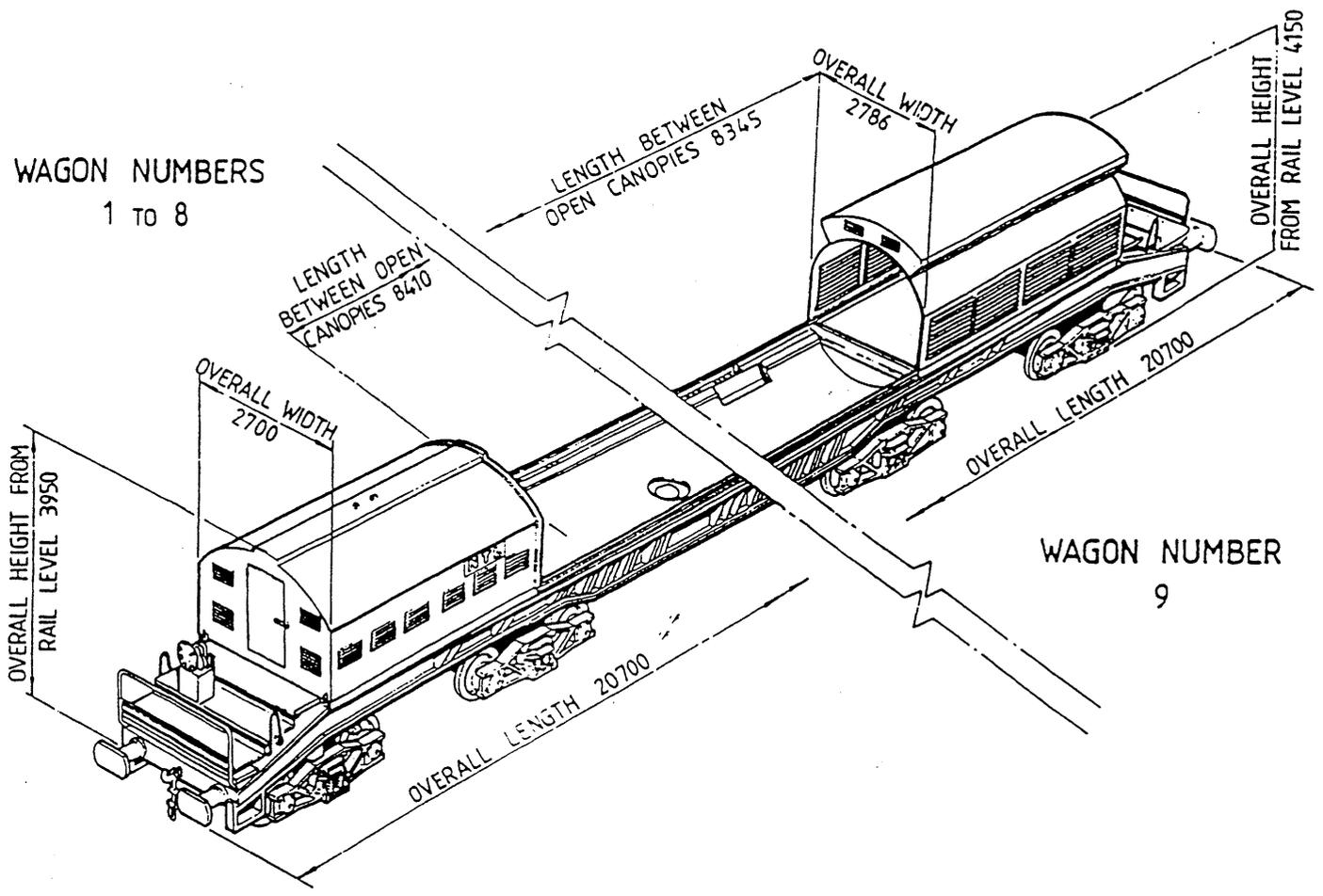
Figure 7.1a: Type of Vehicles being used for Waste Transportation
