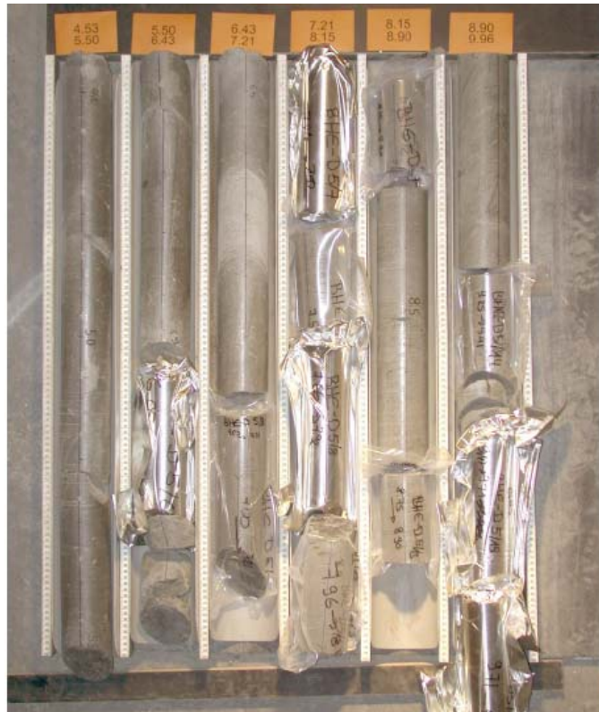
c. Cores drilled from borehole BHE-D5 of D = 84 mm and L = 4.5 - 10.0 m
