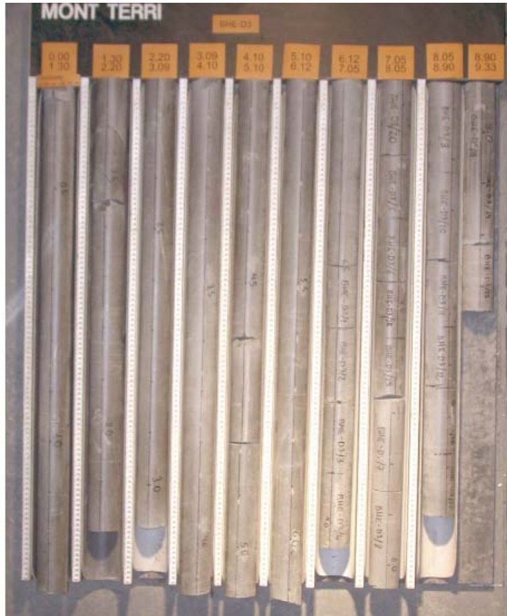
a. Cores drilled from borehole BHE-D3 of D = 62 mm and L = 0 - 9.3 m
