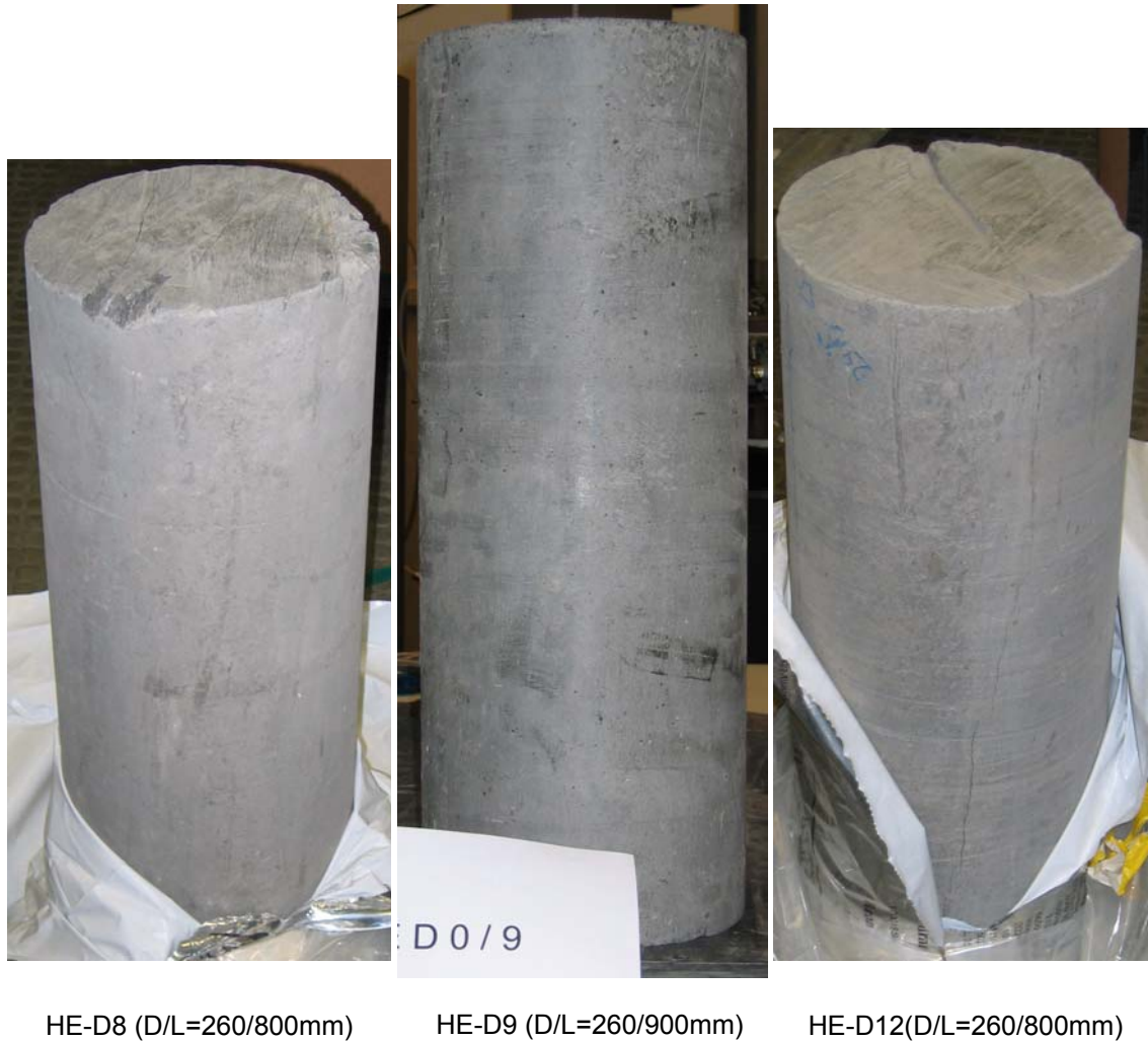
Figure 3-6 Large samples of the Opalinus clay after storage over one year
