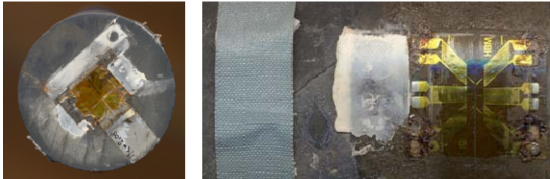
Figure 3-15 Thermally-induced fractures in a sealed Opalinus sample during a heating / cooling cycle between 30 and 73 °C
