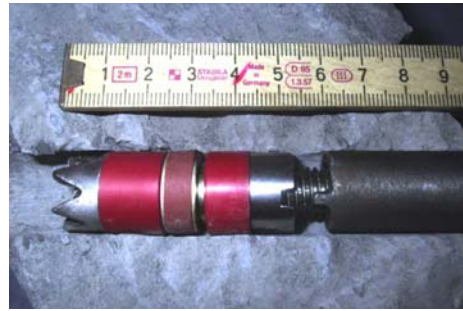
b. Prototype of 20 mm diameter
