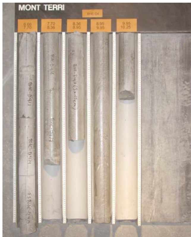
b. Cores drilled from borehole BHE-D4 of D = 84 mm and L = 6.7 - 10.2 m
