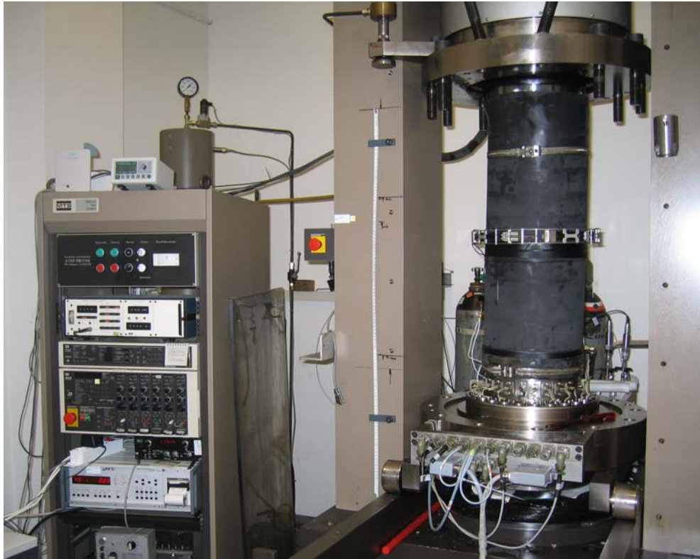
Figure 3-45 Installation of a mock-up heating test in GRS's big triaxial apparatus
