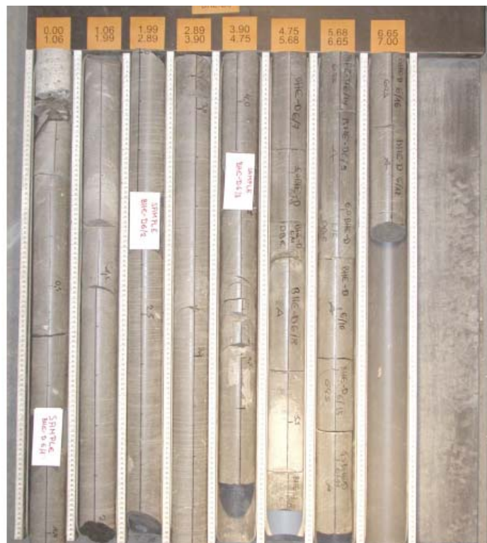
d. Cores drilled from borehole BHE-D6 of D = 72 mm and L = 0 - 7.0 m
