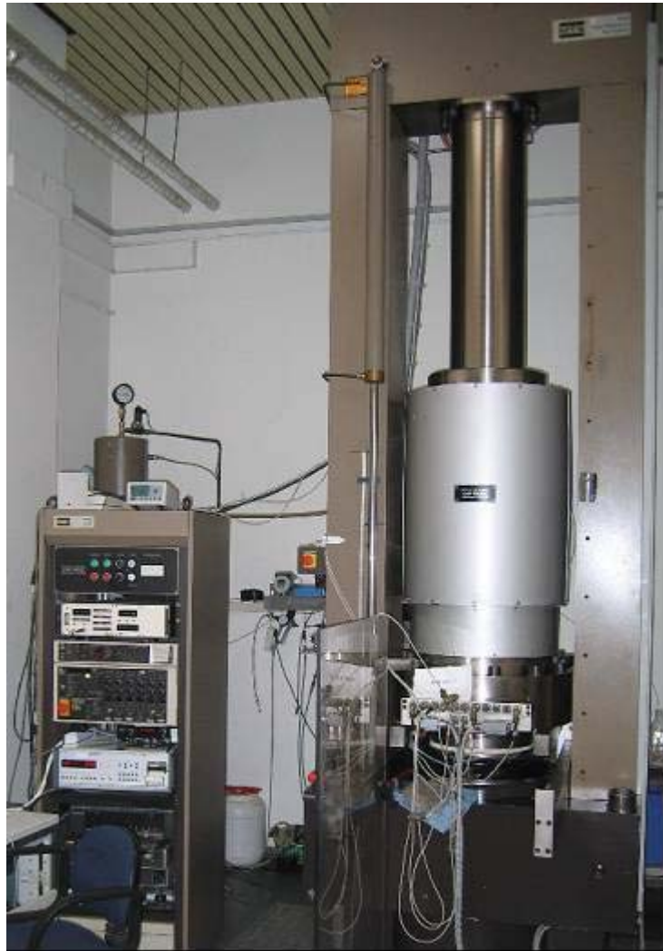
Figure 3-37 Large triaxial apparatus for THM experiments on big samples of 280 mm diameter and 700 mm length
