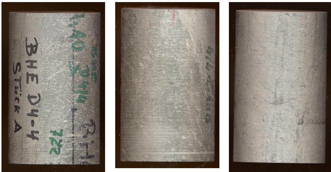
Figure 3-3 Test samples prepared from drilled cores of the Opalinus clay
