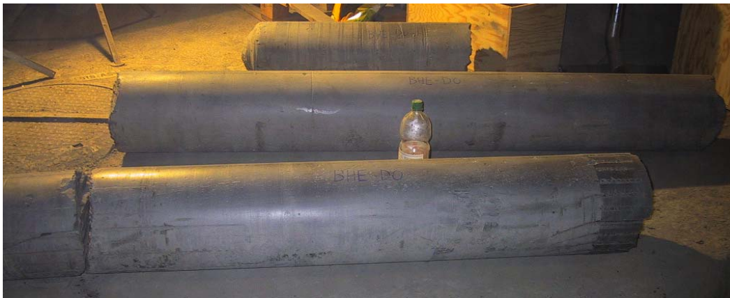
Figure 2-7 Drilled cores (D=260 mm, L=1–2.5 m) from the HE-D heater borehole
