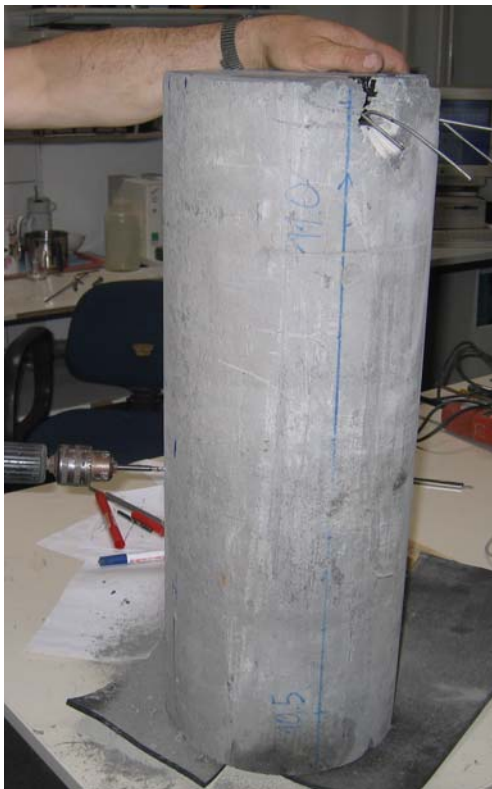
a. borehole drilling
