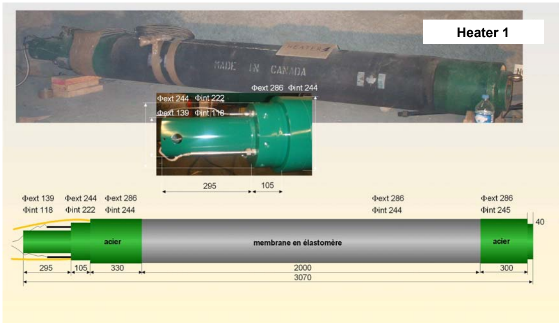
Figure 2-9 Photo and dimension of a HE-D heater
