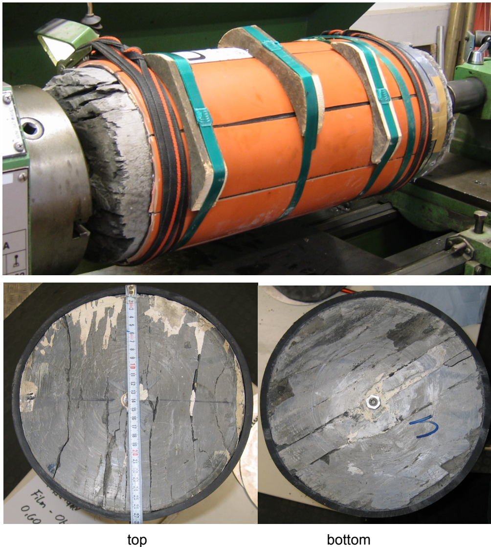
Figure 2.17 Preparation of a large Opalinus clay sample with macro-cracks
