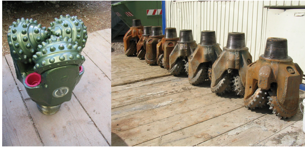
Fig. 3.3 Lateral and front view of a drill bit tool roll used for the rotary method (Source: FRE 3 )
