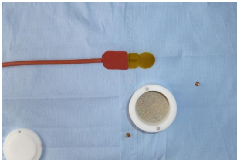
Fig. 3.9 Sample container with SB layer, in red: measurement sensor
