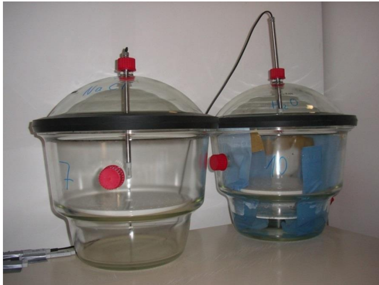
Fig. 3.18 Exsiccators with sensors for temperature and humidity measurement
