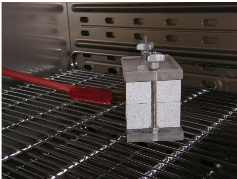
Fig. 3.5 Sample pair in the drying oven (the clamping device is used to assure coupling of sensor to the bentonite)
