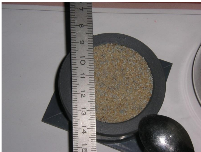
Fig. 3.20 Measurement cell filled with sand/bentonite sample
