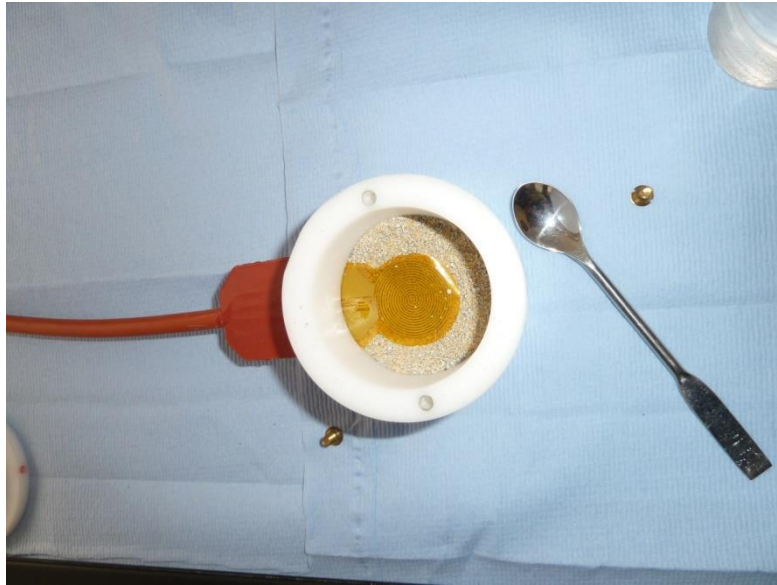
Fig. 3.10 Sensor and SB layer inside the sample container
