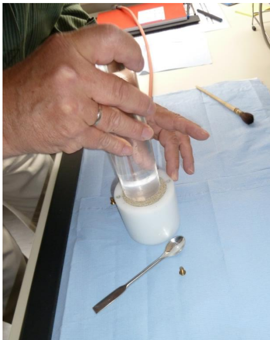
Fig. 3.11 Emplacement of second SB layer into the sample container
