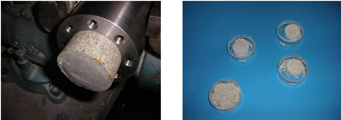
Fig. 3.24 Removal of saturated sand/bentonite from the cell
