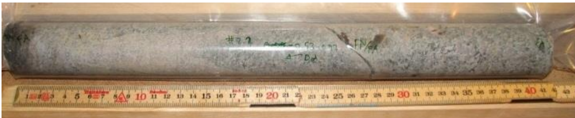
Fig. 5.36 Drill core #2.2 (0.53 – 0.97 m, borehole KA2370A-01) with a natural fracture
