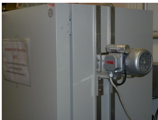
Fig. 7.3 This picture shows a motor fixed at the outside of an oven to exert a gentle rocking motion to the board on which the isopiestic vessels rest
