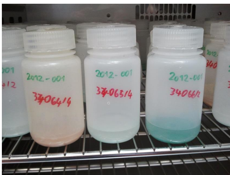
Fig. 7.32 Plastic bottles containing LDH in contact with different salt solutions
