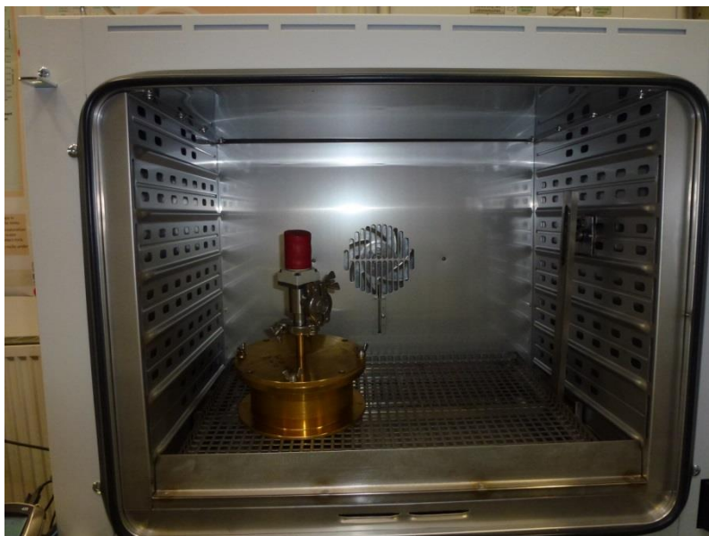
Fig. 7.2 Isopiestic vessel inside an oven
