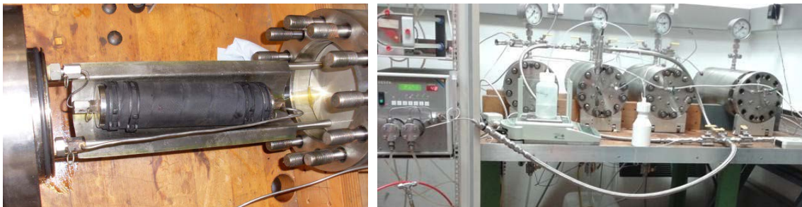
Fig. 3.3 Coated test sample (left); test equipment (right)
