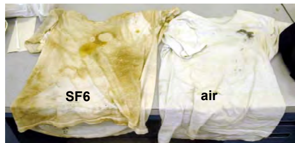
Fig. 6: T-shirt worn by dummy and affected by SF 6 gas (left) and air (right)
