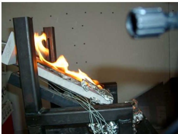
Figure 6 Experimental configuration, PMMA, inclination of 30 °
