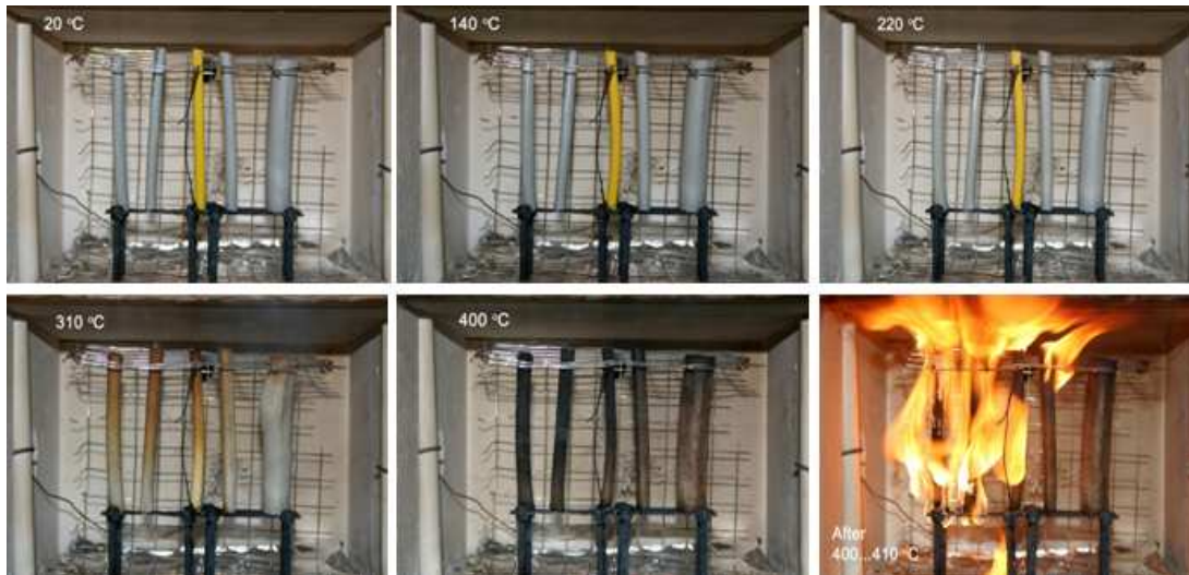
Figure 3 Softening and ignition of I&C cables in a small laboratory furnace
