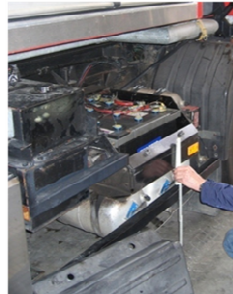
Battery / Air Pressure Tank
